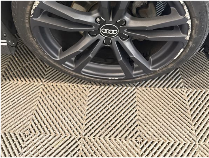
15: Wheel osf Scratched Over 50mm
