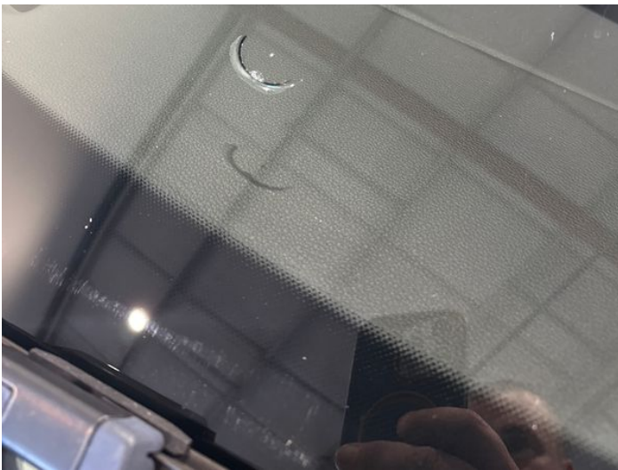
5: Screen Front Cracked Replace
