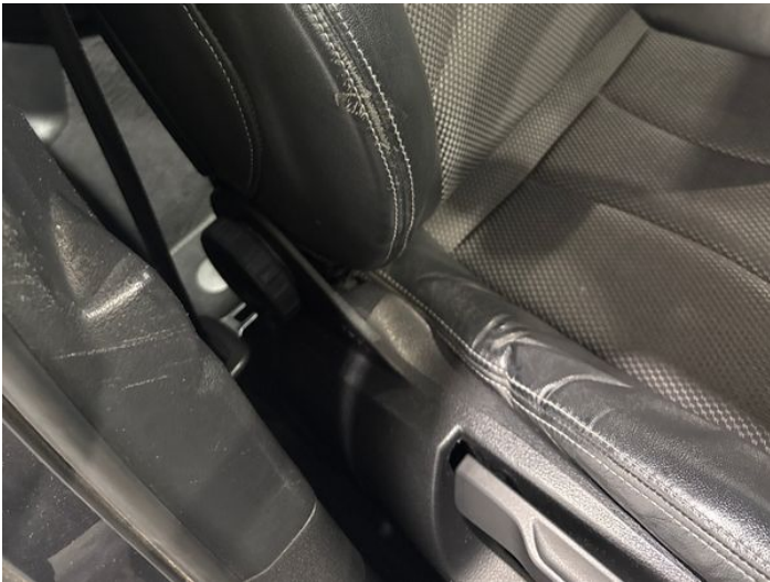
17: Seat Back Cover osf Scuffed Over 25mm
