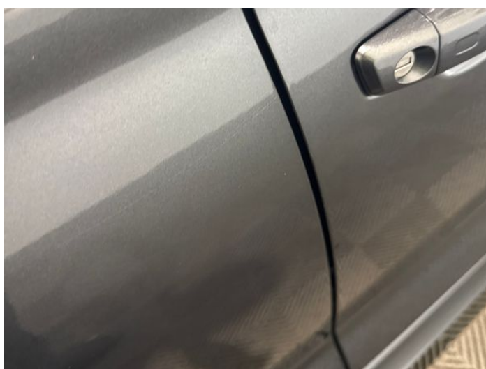
14: Door osr Scratched UpTo 25mm Thru Paint
