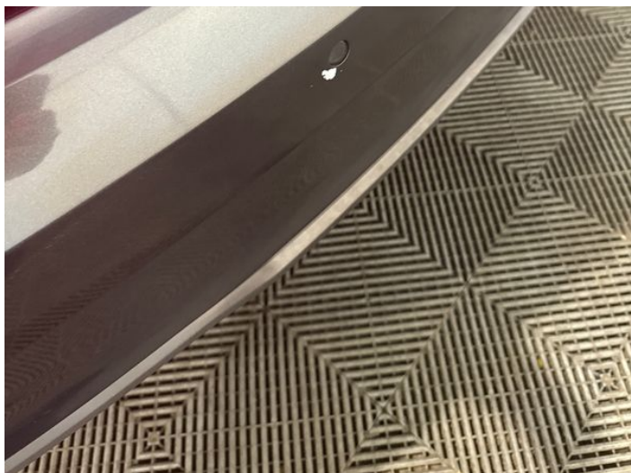
9: Bumper Rear Chipped Over 5mm
