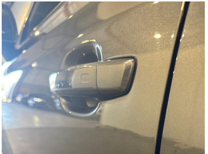
6: Door nsf Dented Between 10mm + 30mm
