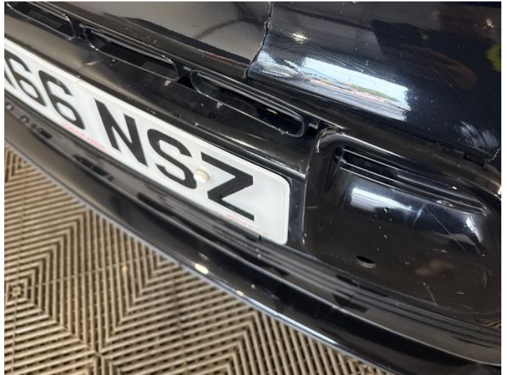
4: Bumper Front Cracked Over 25mm
