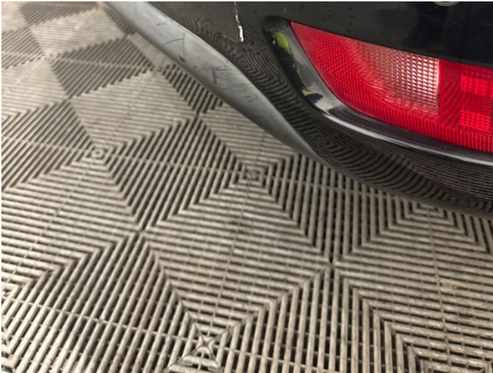
15: Bumper Rear Cracked Over 25mm
