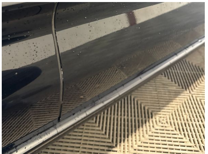
20: Door osf Chipped Edge Chip
