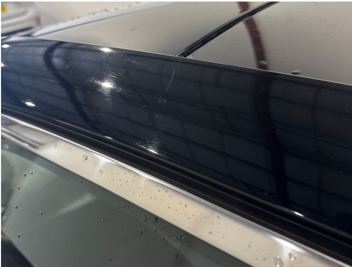
11: A Post ns Scratched UpTo 25mm Thru Paint
