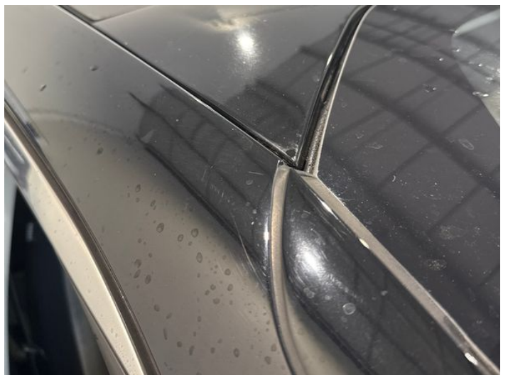
26: Roof Dented Over 30mm
