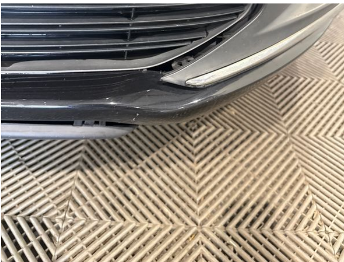
7: Bumper Front Grill Broken Replace
