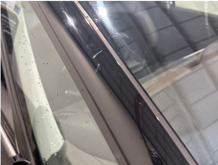
23: A Post os Scratched Over 25mm Thru Paint
