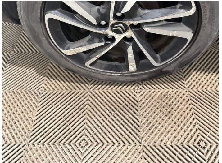
18: Wheel osr Scratched Over 50mm
