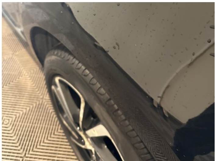
14: Qtr Panel nsr Dented Over 30mm
