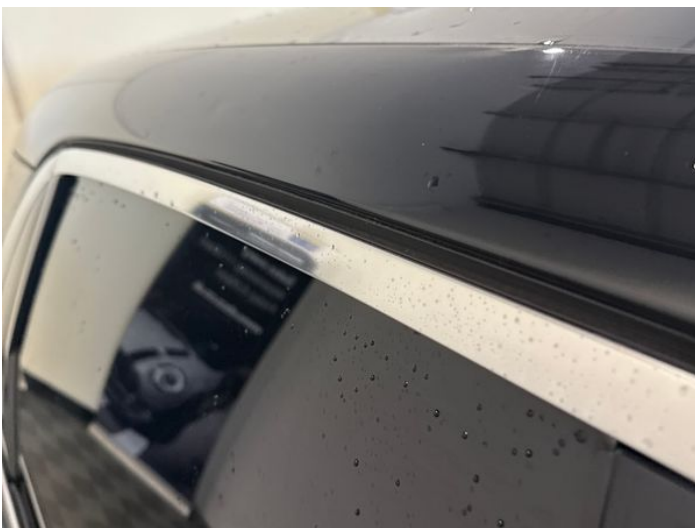
25: B Post os Dented Between 10mm + 30mm
