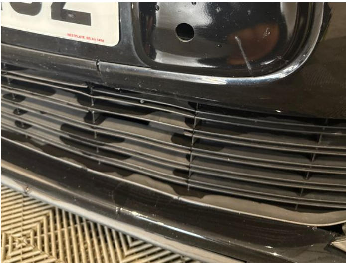
5: Parking Sensor Front Missing Replace
