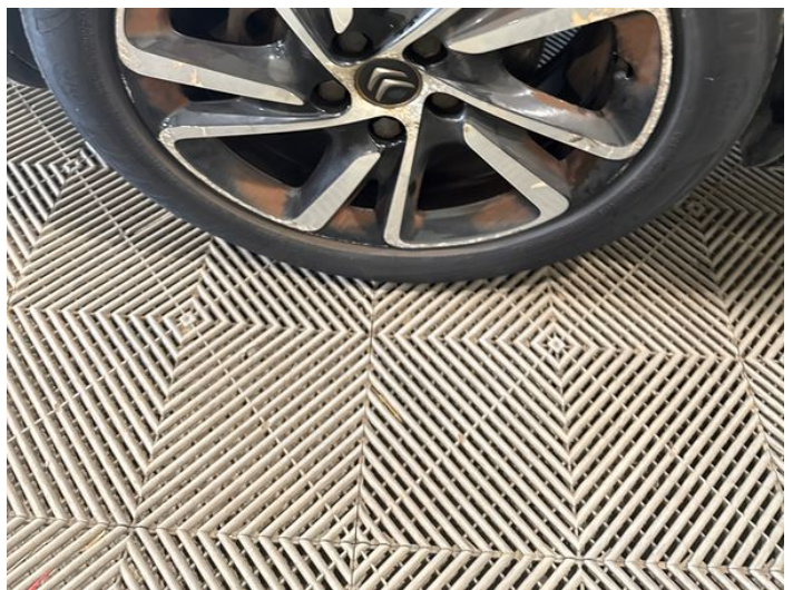
8: Wheel nsf Scratched Over 50mm
