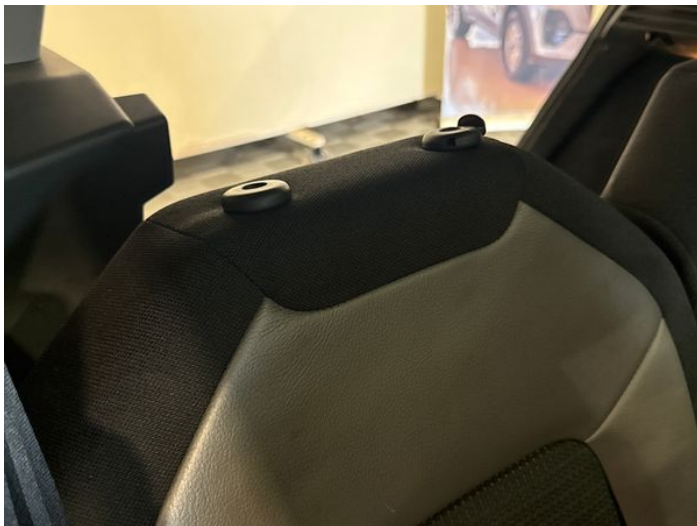
1: Headrest Assy Rear Seat os Missing Replace
