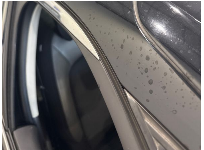
24: A Post os Dented Between 10mm + 30mm
