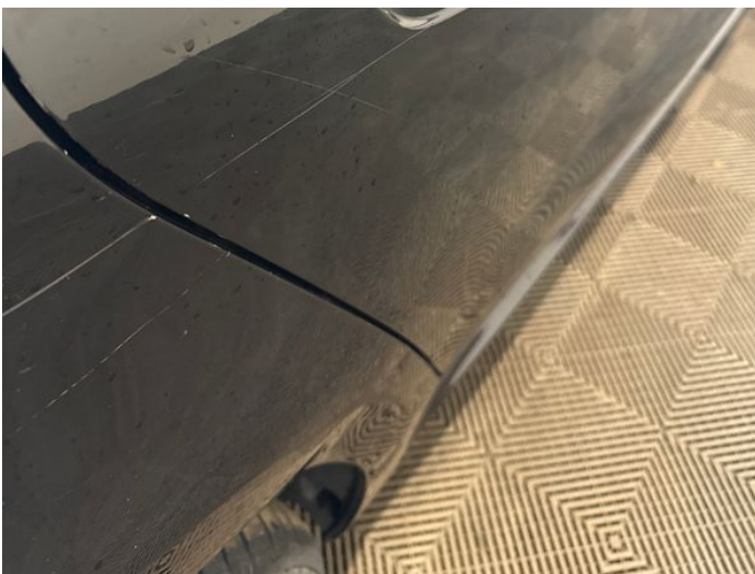
19: Door osr Scratched Over 25mm Thru Paint
