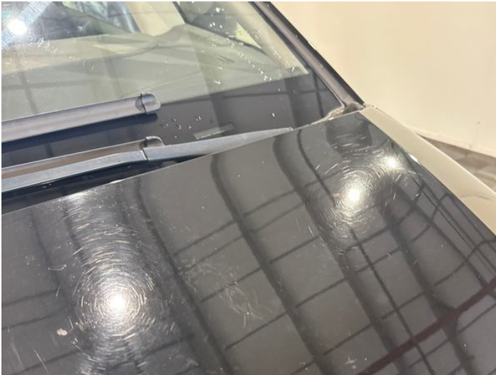
3: Bonnet Scratched Over 25mm Thru Paint
