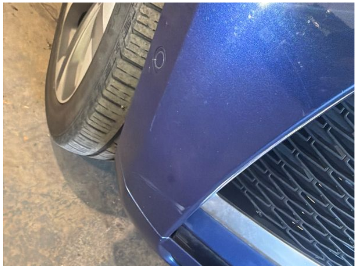
6: Bumper Front Scratched 25 to 100mm Thru Paint
