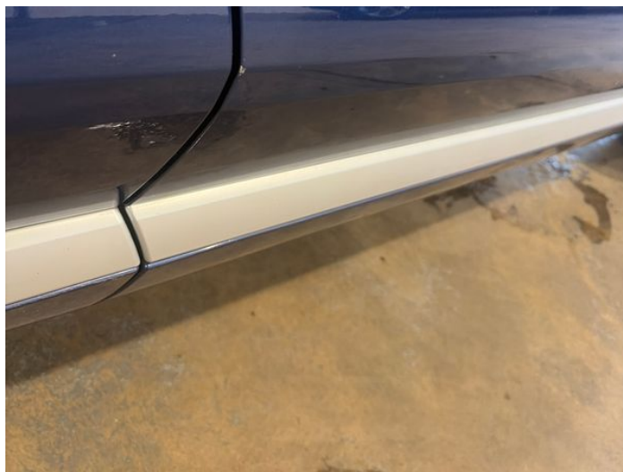
2: Door osf Chipped Edge Chip
