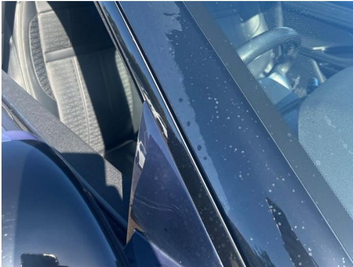
4: A Post os Poor Previous Repair Poor Paint
