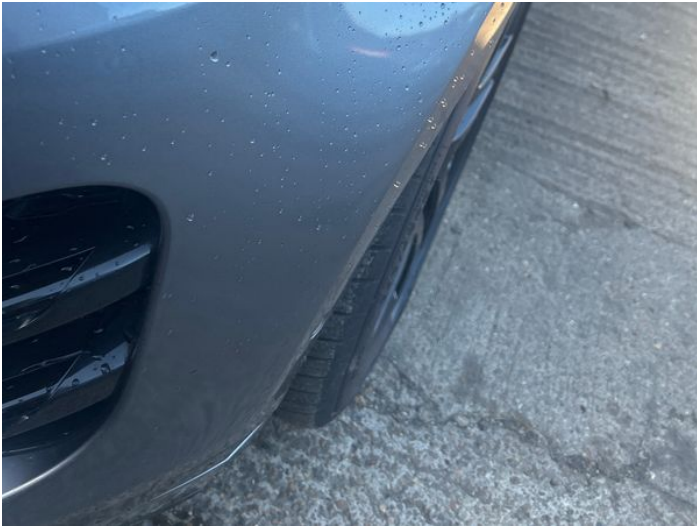
3: Bumper Front Poor Previous Repair Poor Paint
