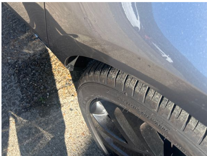
1: Wing osf Poor Previous Repair Poor Paint
