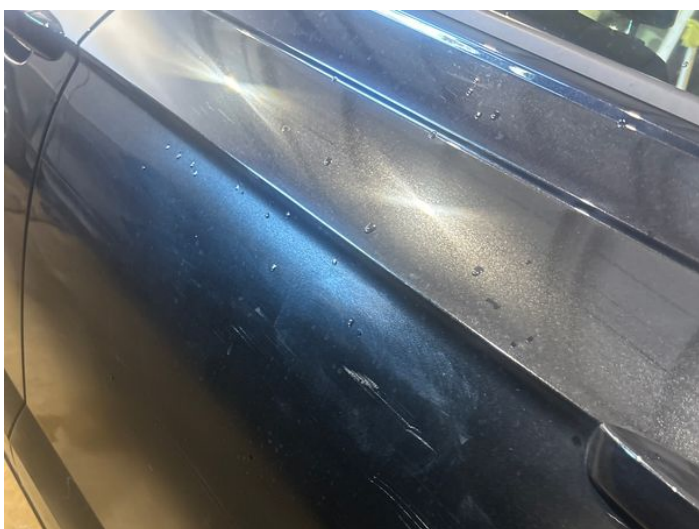
11: Door nsr Poor Previous Repair Poor Paint
