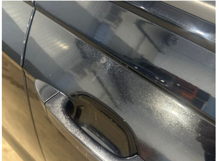
4: Door osf Poor Previous Repair Poor Paint
