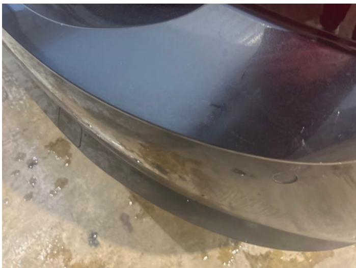
9: Bumper Rear Poor Previous Repair Poor Paint
