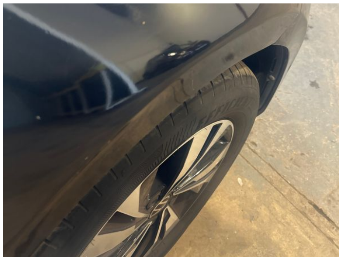
2: Wing osf Poor Previous Repair Poor Paint
