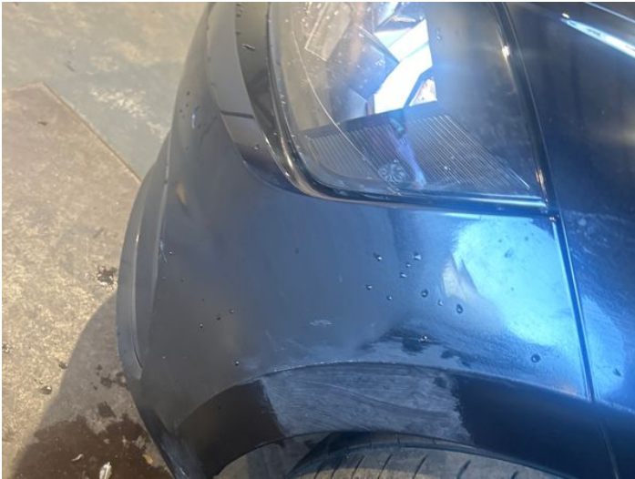
15: Bumper Front Poor Previous Repair Poor Paint
