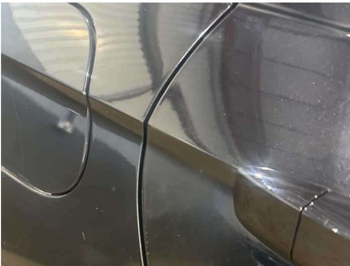
5: Door osr Poor Previous Repair Poor Paint
