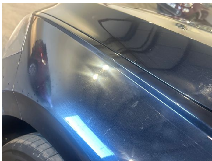
14: Wing nsf Poor Previous Repair Poor Paint
