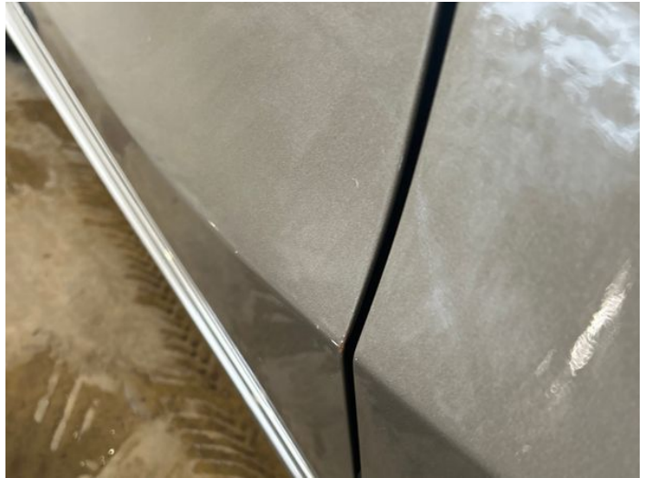
10: Door nsf Chipped Edge Chip
