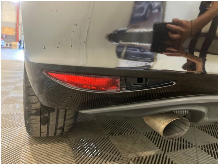
11: Reflector nsr Broken Replace
