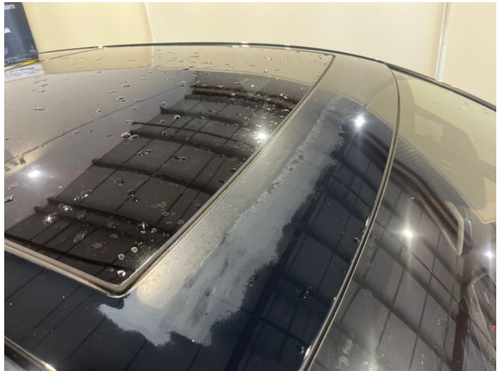
12: Roof Scratched Over 25mm Thru Paint
