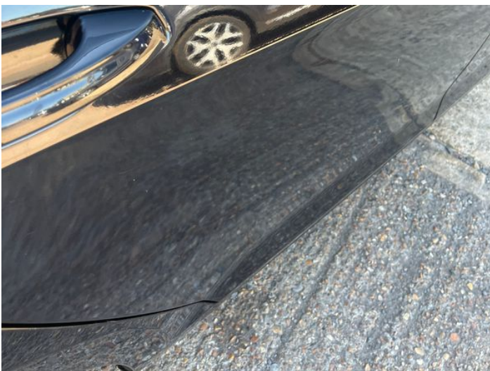
13: Door osr Poor Previous Repair Poor Paint
