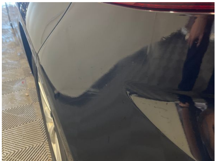
8: Bumper Rear Poor Previous Repair Poor Paint
