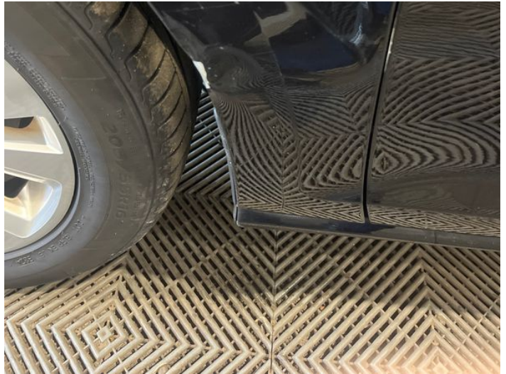
4: Wing nsf Dented With Paint Damage
