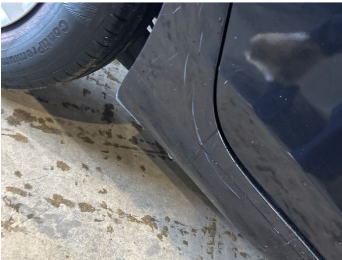
5: Sill os Scratched Over 25mm Thru Paint
