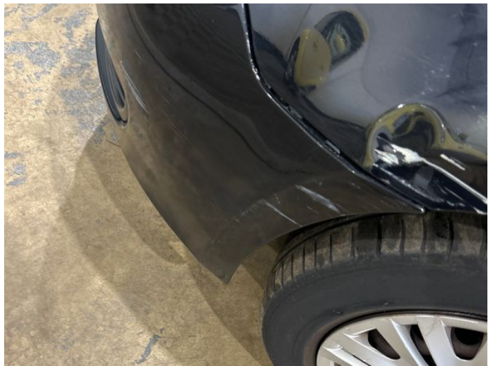
12: Bumper Front Scratched Over 100mm Thru Paint
