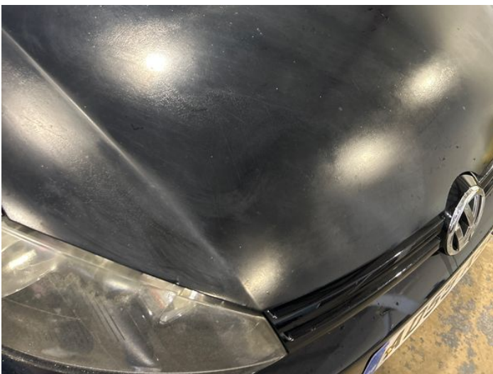
13: Bonnet Poor Previous Repair Poor Paint
