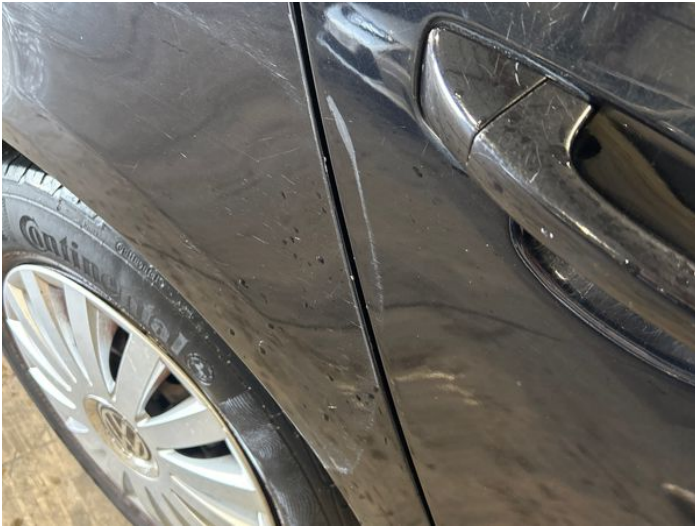
3: Door osr Scratched Over 25mm Thru Paint
