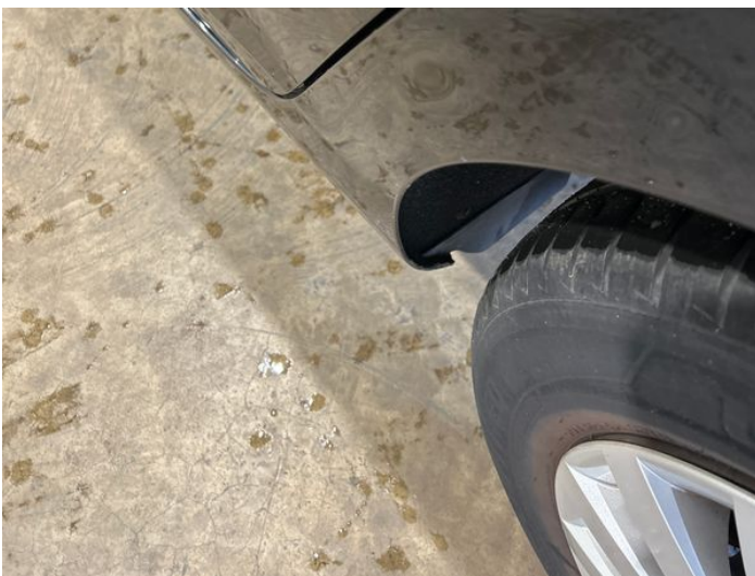
7: Qtr Panel nsr Dented Between 10mm + 30mm
