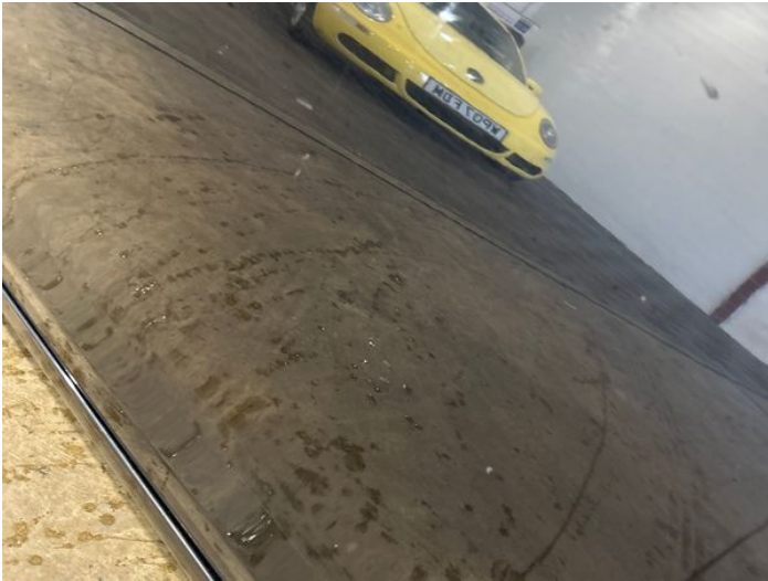
9: Door nsf Chipped Multiple Chips
