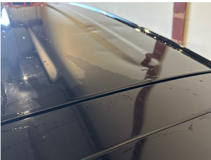
13: Roof Dented Over 30mm
