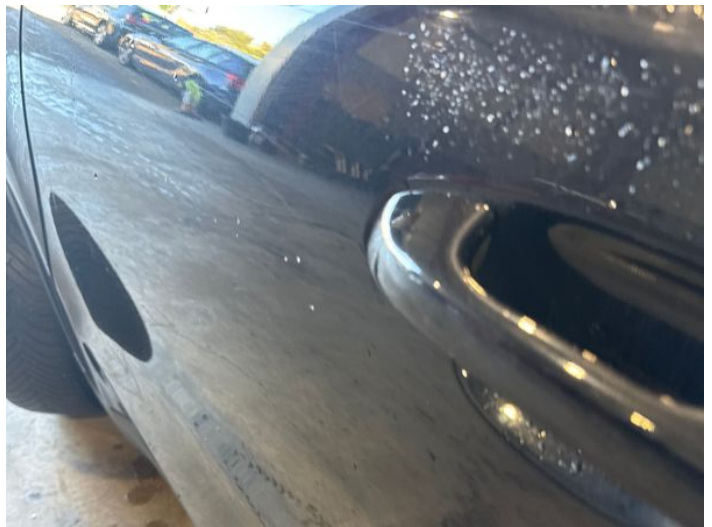
6: Door nsf Chipped Multiple Chips
