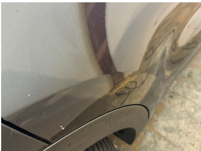
17: Door osr Scratched Over 25mm Thru Paint
