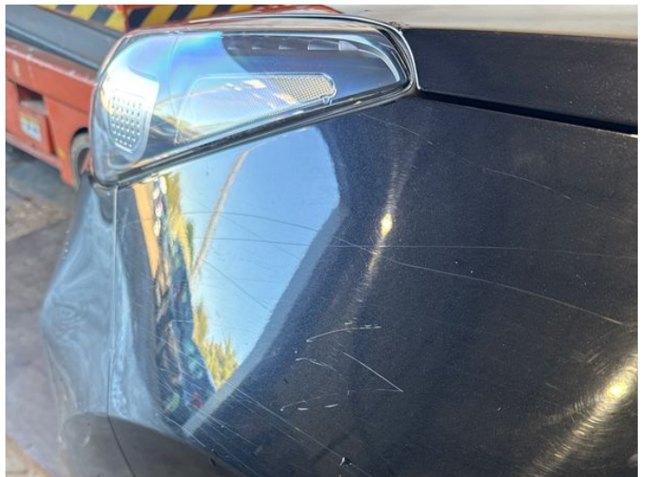
4: Wing nsf Scratched Over 25mm Thru Paint
