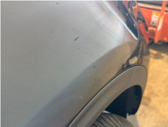
21: Wing osf Scratched UpTo 25mm Thru Paint
