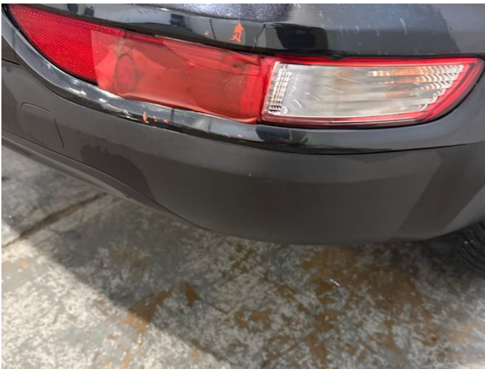
11: Bumper Reflector osr Broken Replace
