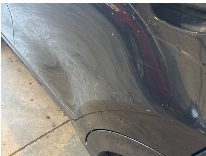
7: Door nsr Scratched Over 25mm Thru Paint
