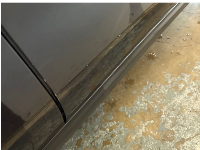
19: Door osf Scratched Over 25mm Thru Paint
