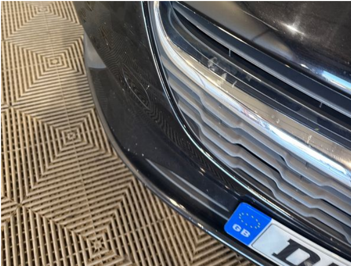
3: Bumper Front Scratched Over 100mm Thru Paint
