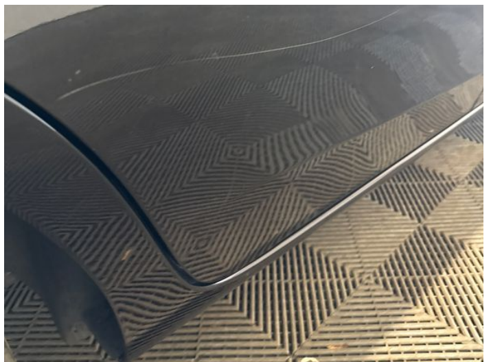
14: Door osr Scratched Over 25mm Thru Paint
