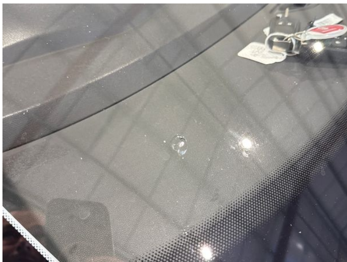
1: Screen Front Chipped Over 10mm
