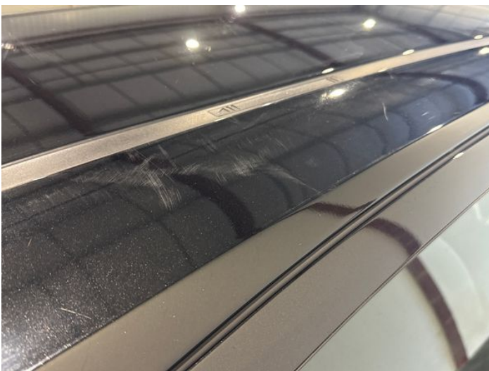
13: B Post os Scratched Over 25mm Thru Paint
