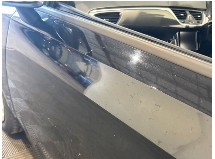
6: Door nsf Scratched Over 25mm Thru Paint
