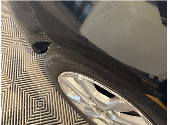
4: Wing nsf Scratched UpTo 25mm Thru Paint
