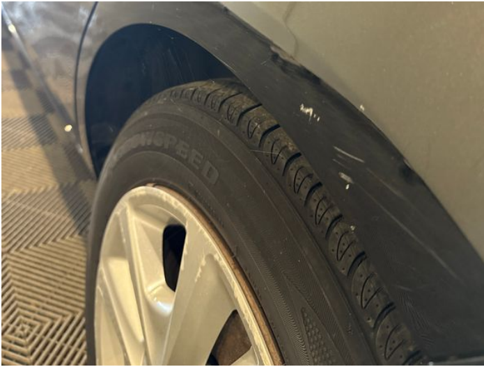
9: Qtr Panel nsr Dented Between 10mm + 30mm
