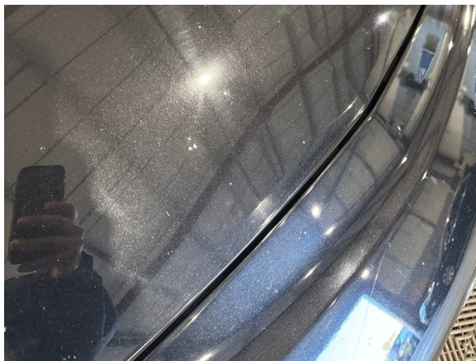
2: Bonnet Scratched Over 25mm Thru Paint
