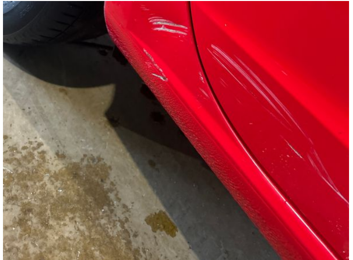
4: Sill os Dented With Paint Damage
