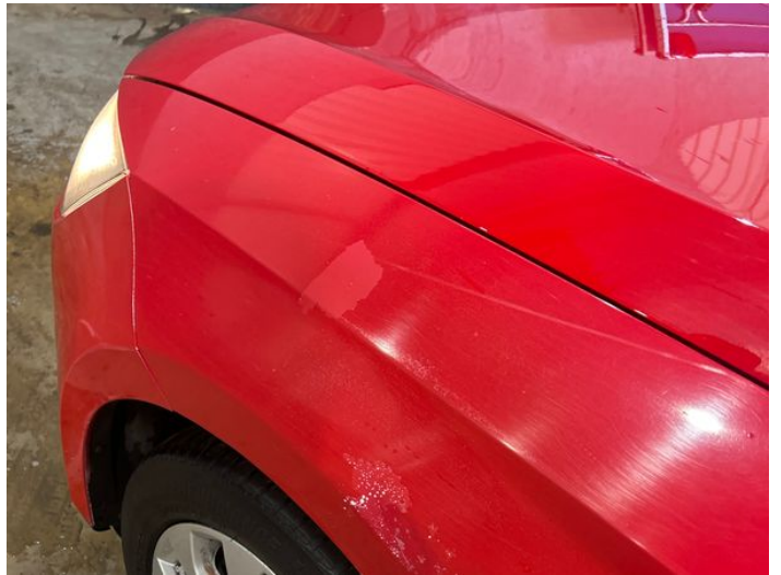
12: Wing nsf Poor Previous Repair Paint Flake
