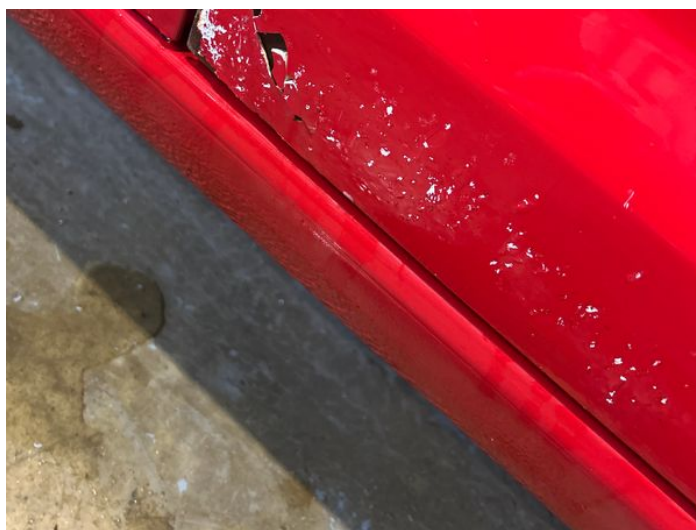
2: Door osf Poor Previous Repair Paint Flake
