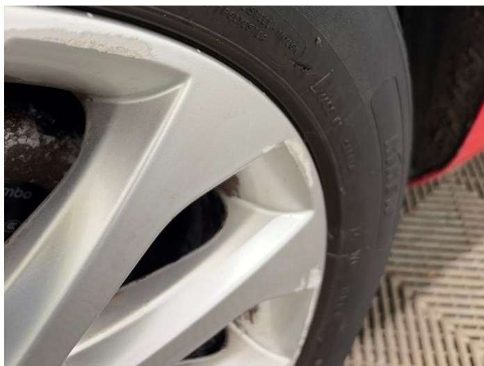
18: Tyre osr Damaged Replace
