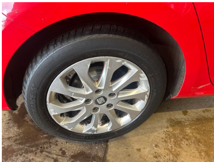
16: Wheel osr Scratched Over 50mm
