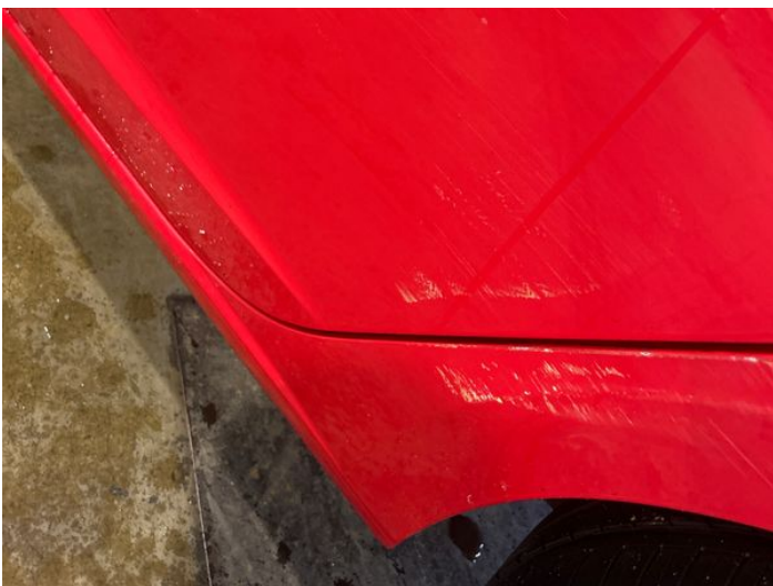
7: Door nsr Scratched Over 25mm Thru Paint
