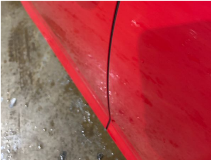
9: Door nsf Chipped Edge Chip
