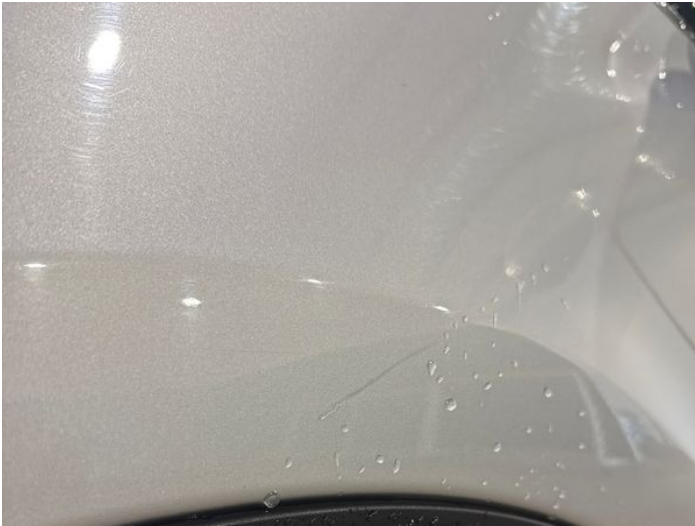
3: Wing nsf Scratched Over 25mm Thru Paint
