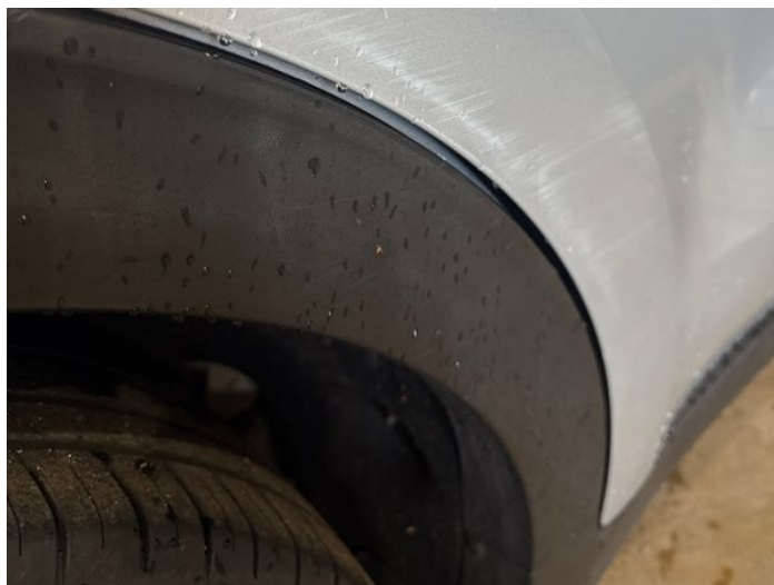
10: Door osr Scratched Over 25mm Thru Paint
