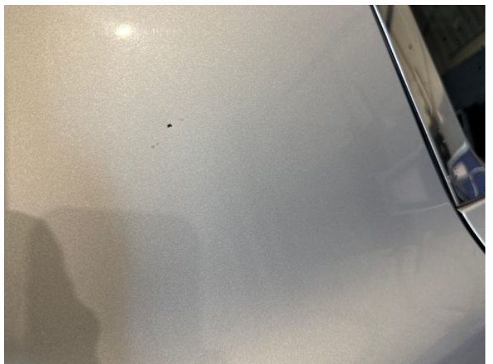
8: Qtr Panel osr Chipped 1 To 5
