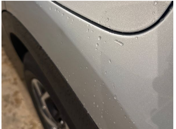
6: Qtr Panel nsr Dented Between 10mm + 30mm
