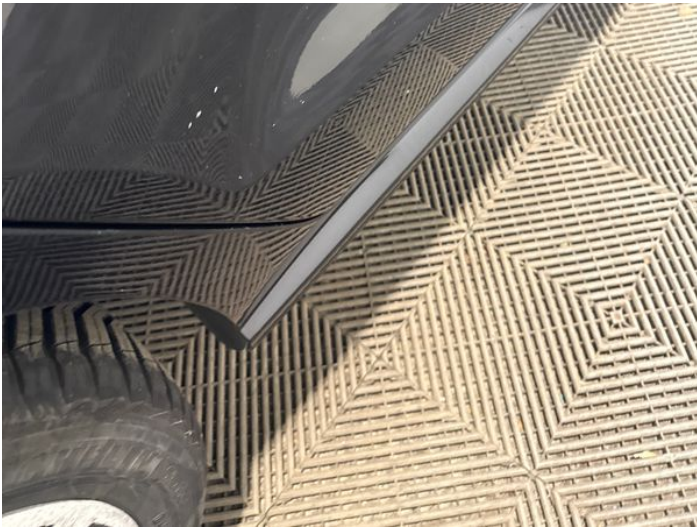
17: Door osr Chipped Multiple Chips
