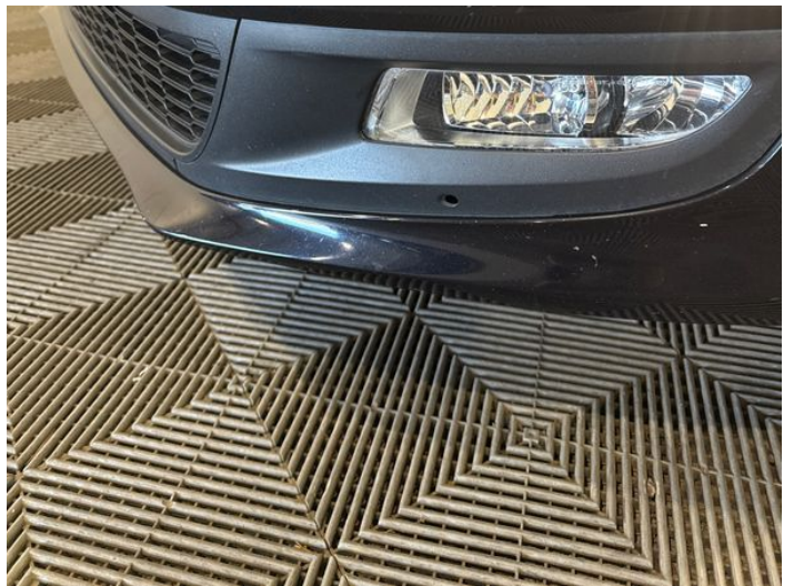
2: Bumper Front Poor Previous Repair Poor Paint
