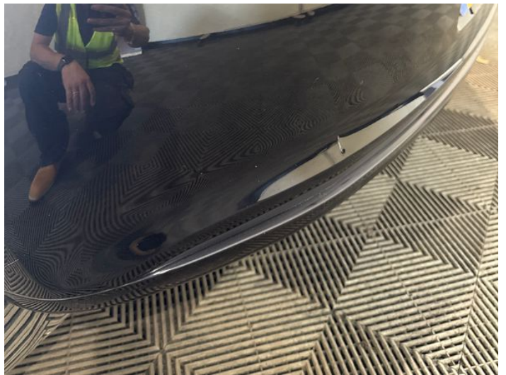
12: Bumper Rear Cracked UpTo 25mm
