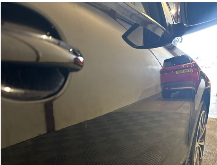
19: Door osf Dented 2 Or Less UpTo 10mm
