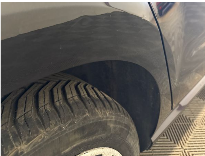
13: Qtr Panel osr Dented Over 2 UpTo 10mm
