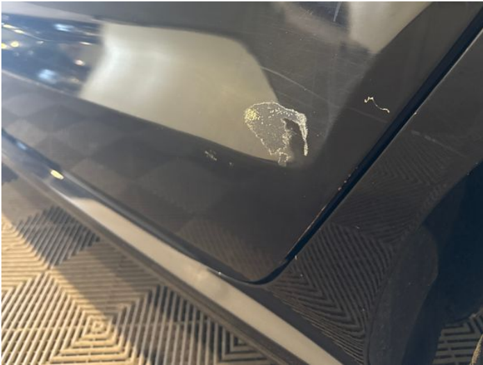
9: Door nsr Dented With Paint Damage
