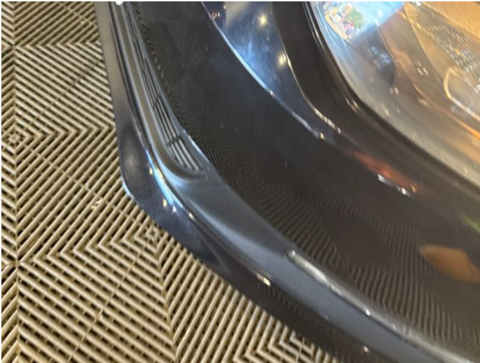
3: Bumper Front Chipped Multiple Chips
