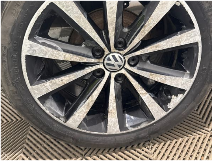
15: Wheel osr Scratched Over 50mm
