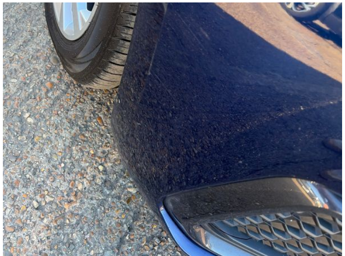
10: Bumper Front Scratched 25 to 100mm Thru Paint
