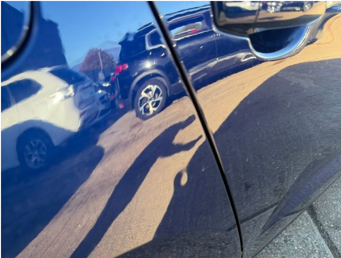
3: Qtr Panel osr Dented Between 10mm + 30mm
