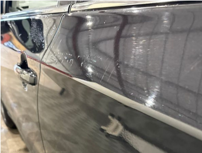
9: Door nsr Dented Between 10mm + 30mm
