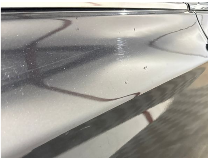
13: Door osr Scratched UpTo 25mm Thru Paint
