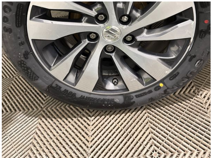
12: Wheel osr Scratched Over 50mm
