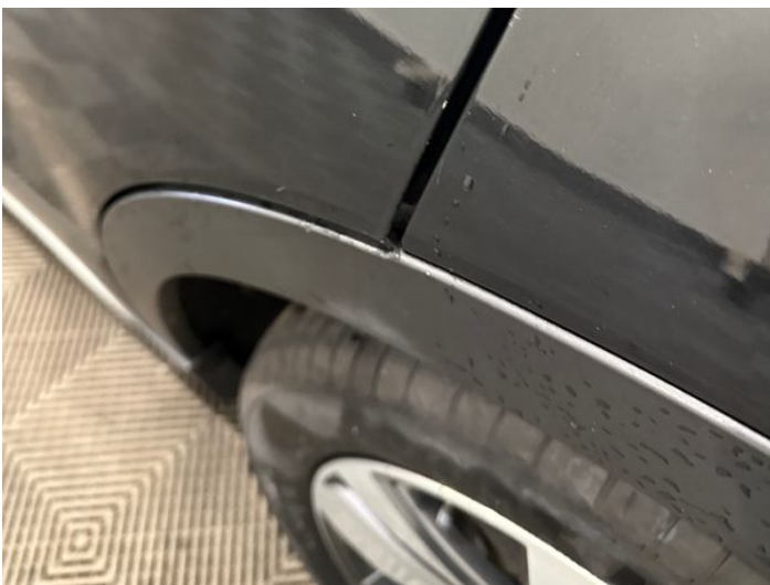
7: Door nsr Chipped Edge Chip
