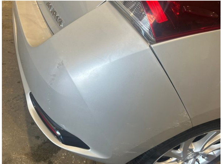
4: Bumper Rear Poor Previous Repair Poor Paint
