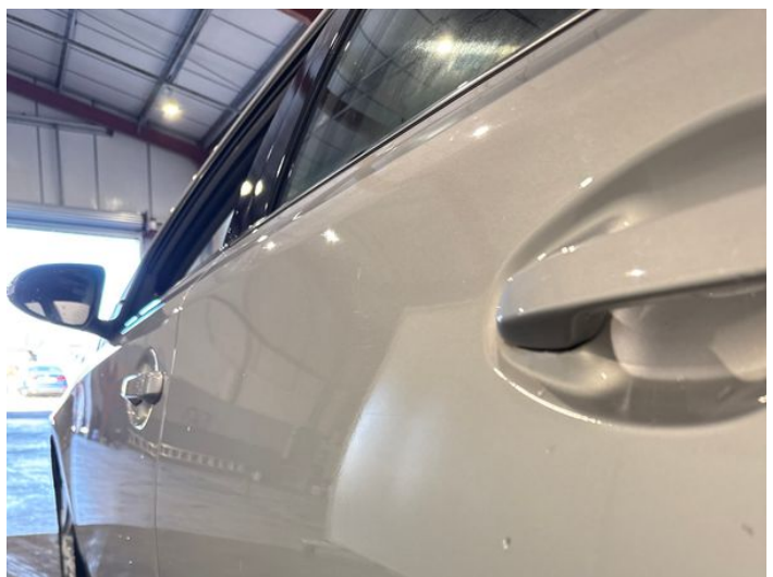
12: Door nsr Poor Previous Repair Rippled UpTo 30%
