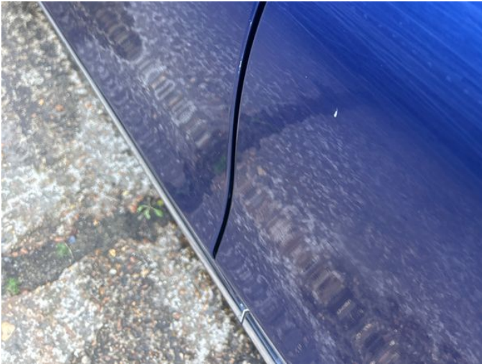
15: Door nsf Chipped Edge Chip
