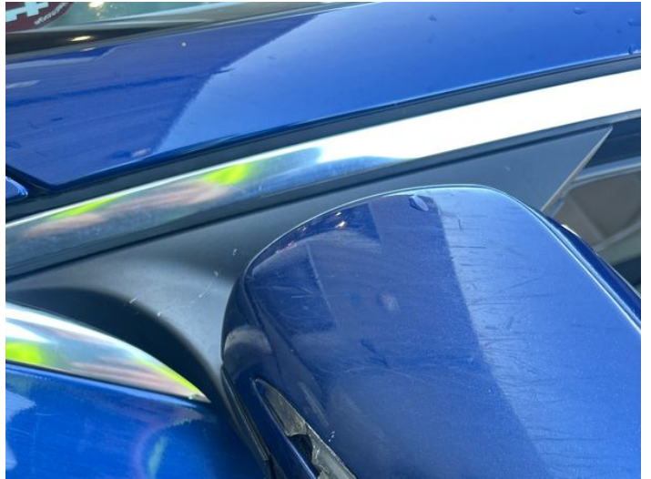
16: Door Mirror Assy nsf Broken Replace
