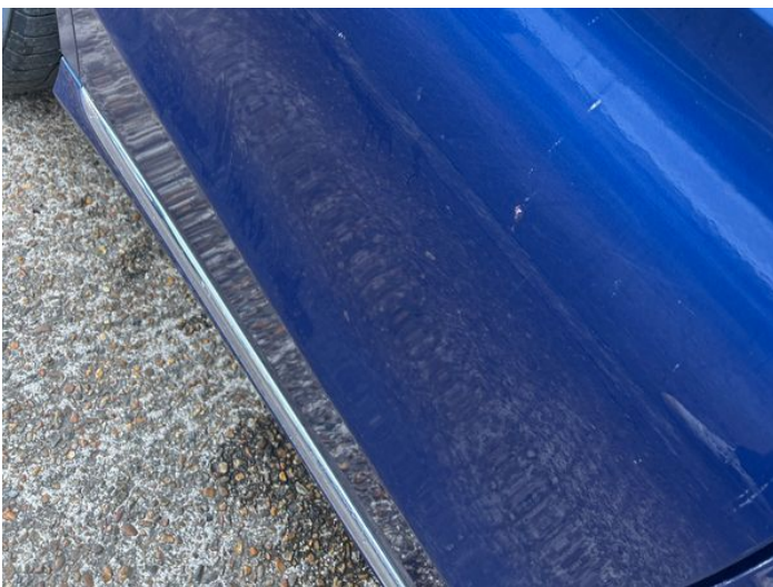
7: Door osr Chipped Multiple Chips
