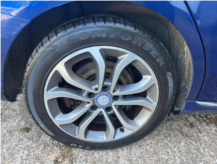
3: Wheel osr Scratched Over 50mm
