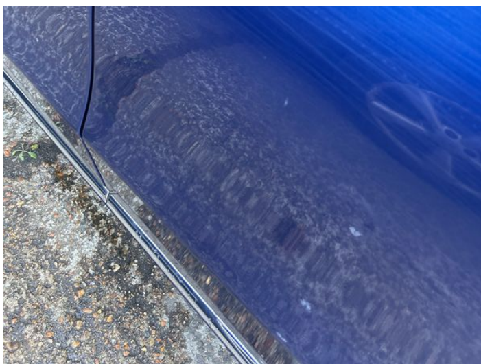
13: Door nsr Chipped 1 To 5
