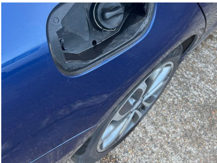
11: Fuel Flap Missing Replace
