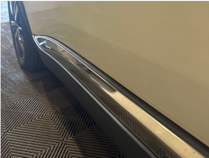
5: Door nsf Dented With Paint Damage
