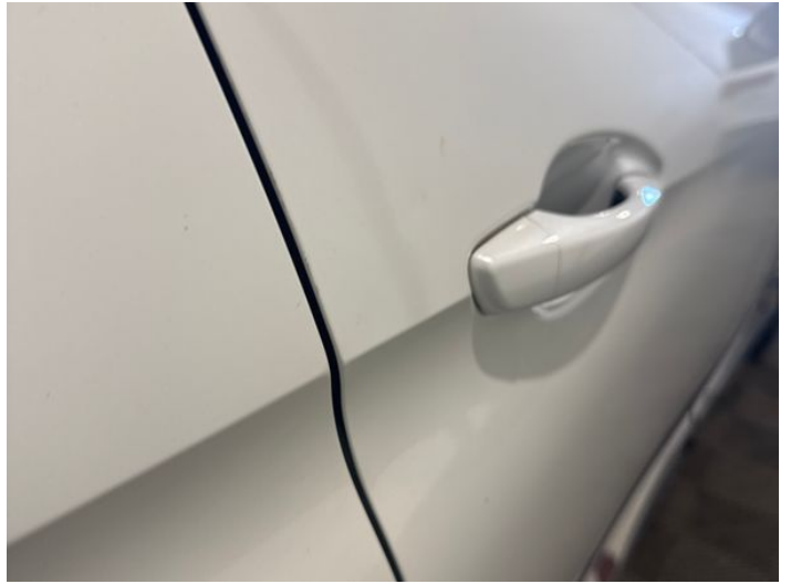
10: Door osr Dented Between 10mm + 30mm
