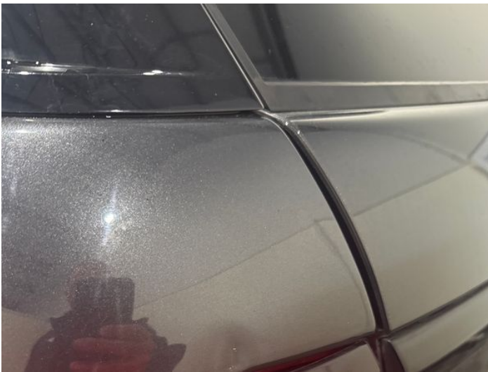
11: Qtr Panel nsr Dented Between 10mm + 30mm
