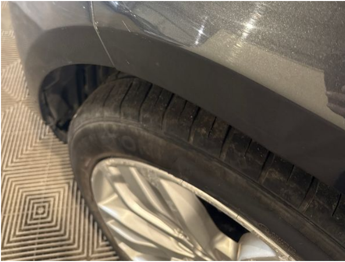
3: Wing nsf Dented Over 30mm
