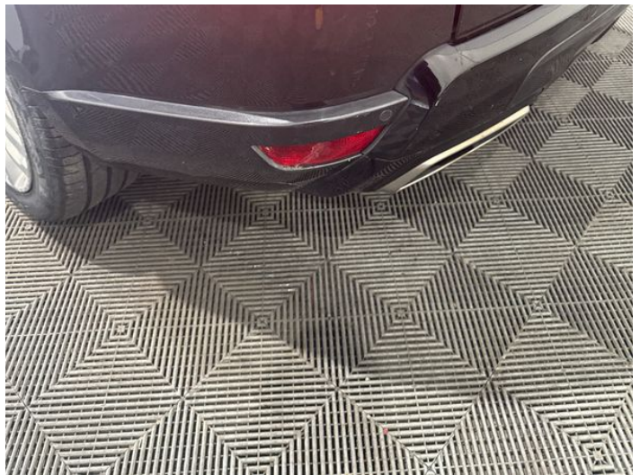
12: Bumper Rear Moulding Scratched (Painted) Over 25mm Thru Paint
