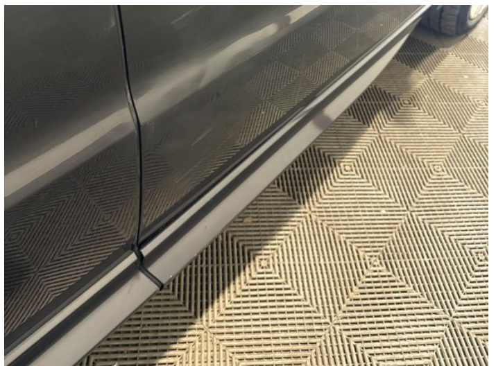
20: Door osf Dented With Paint Damage
