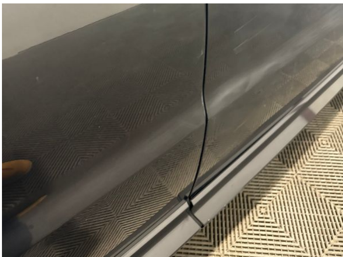
21: Door osr Scratched Over 25mm Thru Paint
