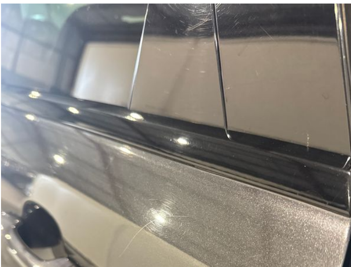
7: Door nsr Scratched Over 25mm Thru Paint
