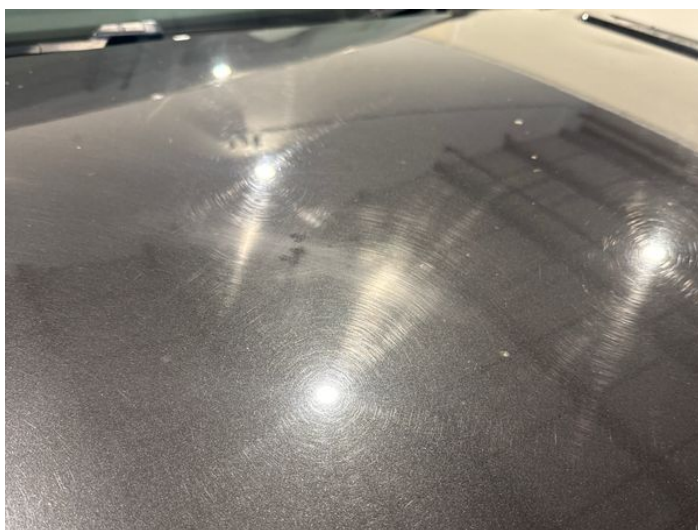
1: Bonnet Scratched Over 25mm Thru Paint
