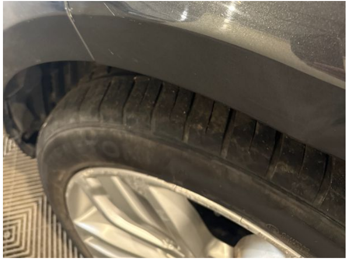
4: Wing nsf Scratched UpTo 25mm Thru Paint
