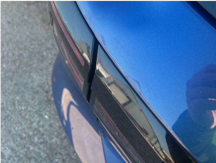
17: Tailgate Dented With Paint Damage
