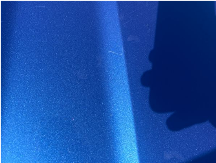
15: Bonnet Scratched UpTo 25mm Thru Paint
