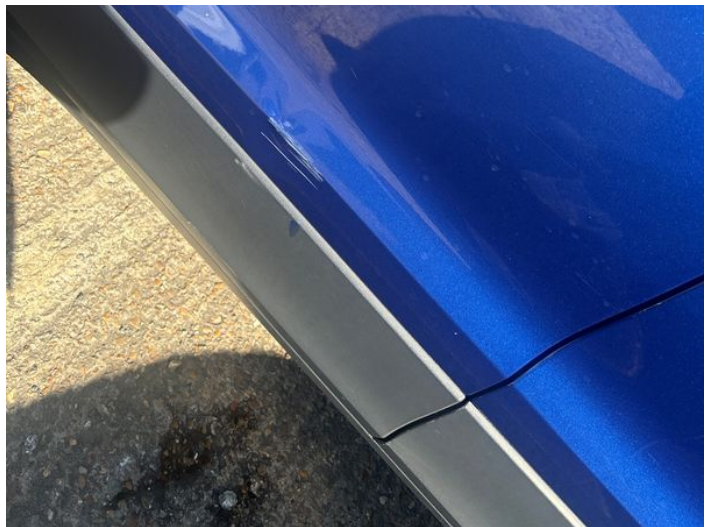
4: Door osr Scratched Over 25mm Thru Paint
