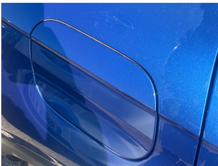
7: Qtr Panel osr Scratched UpTo 25mm Thru Paint
