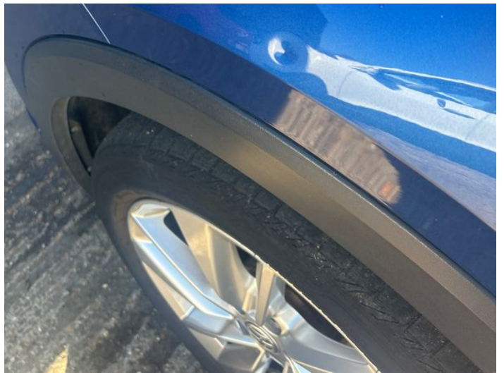
12: Wing nsf Dented Between 10mm + 30mm
