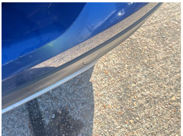
8: Bumper Rear Poor Previous Repair Poor Paint
