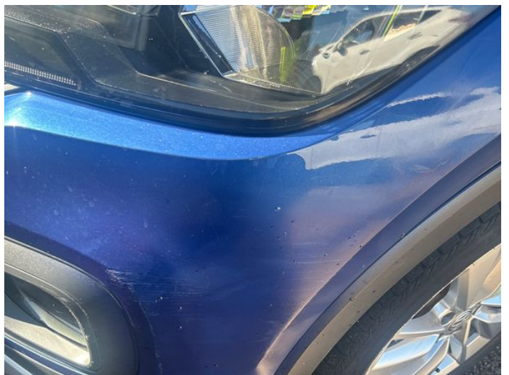
14: Bumper Front Poor Previous Repair Poor Paint
