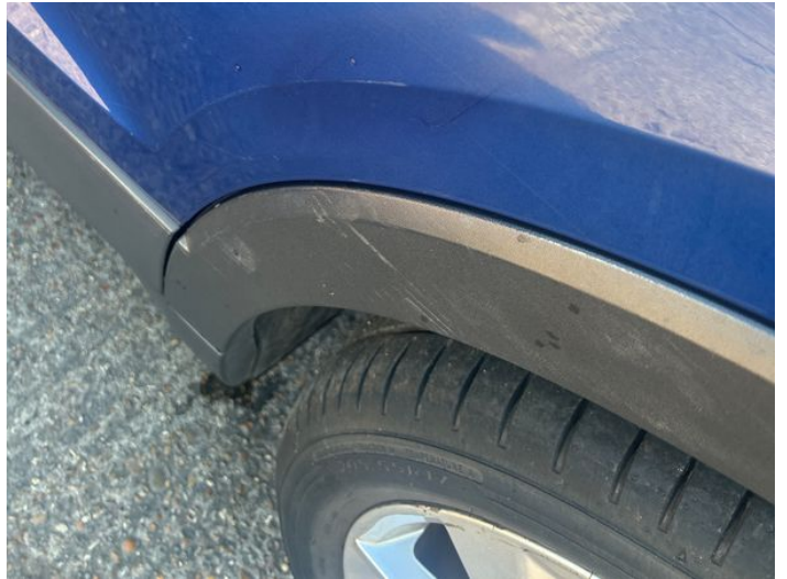
10: Door nsr Poor Previous Repair Poor Paint
