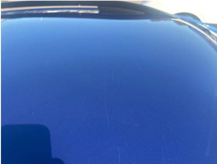
16: Roof Scratched Over 25mm Thru Paint
