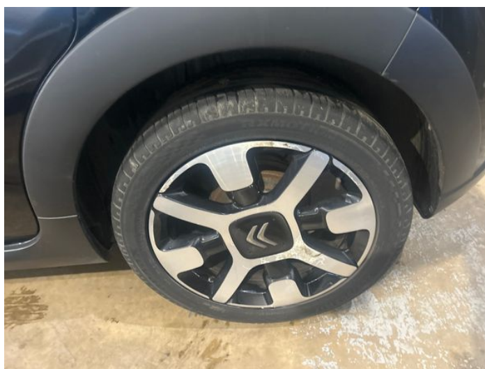
6: Wheel nsr Corroded Light
