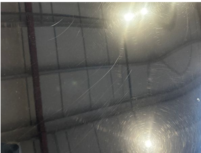
13: Bonnet Scratched Over 25mm Thru Paint
