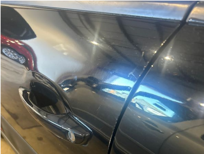
9: Door nsf Chipped Edge Chip
