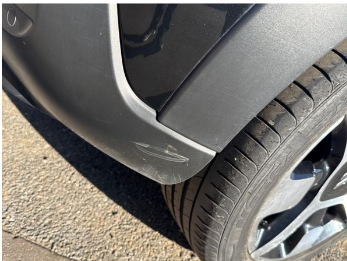
15: Bumper Rear Moulding Scuffed (Unpainted) UpTo 100mm
