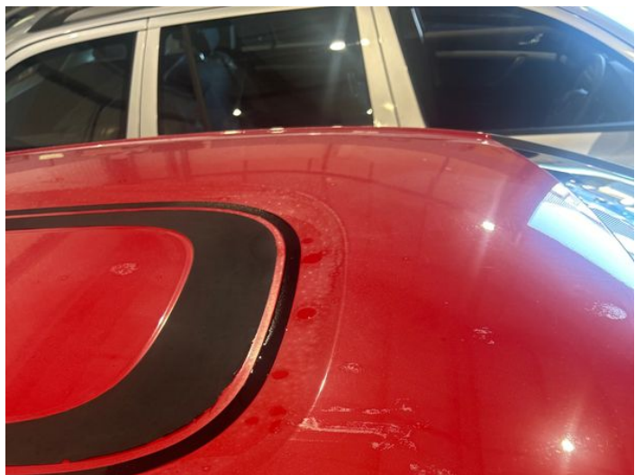
14: Roof Poor Previous Repair Paint Flake
