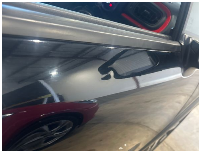
2: Door osf Dented Over 30mm
