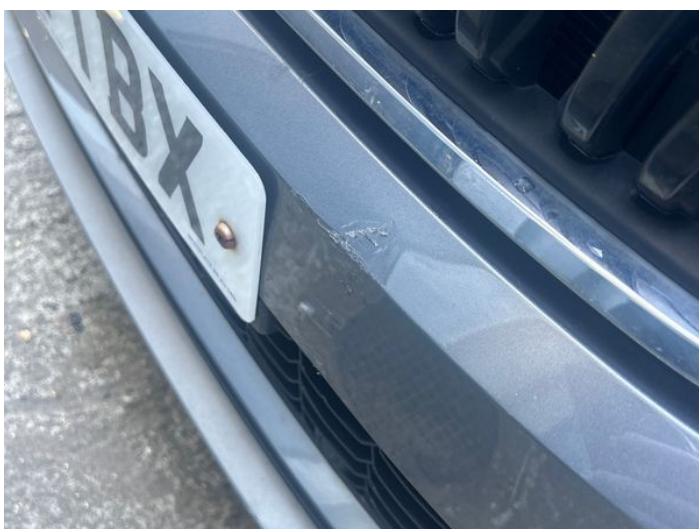
17: Bumper Front Dented With Paint Damage
