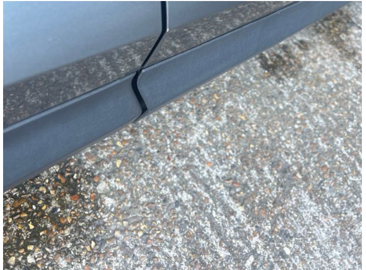
4: Door osf Chipped Edge Chip
