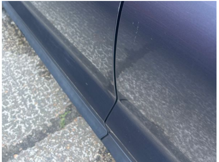
12: Door nsf Chipped Edge Chip
