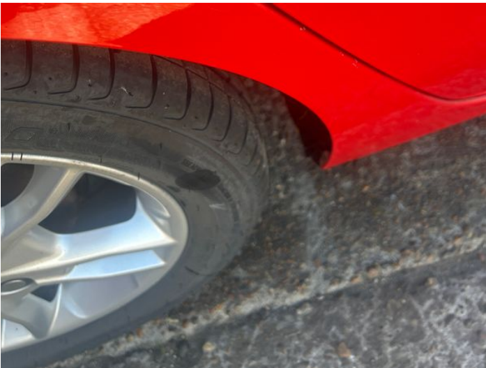
8: Qtr Panel osr Chipped 1 To 5
