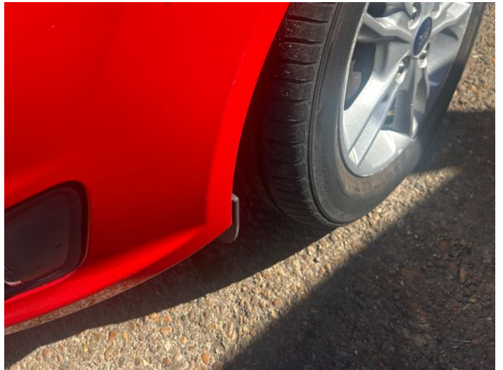
18: Bumper Front Scratched Over 100mm Thru Paint
