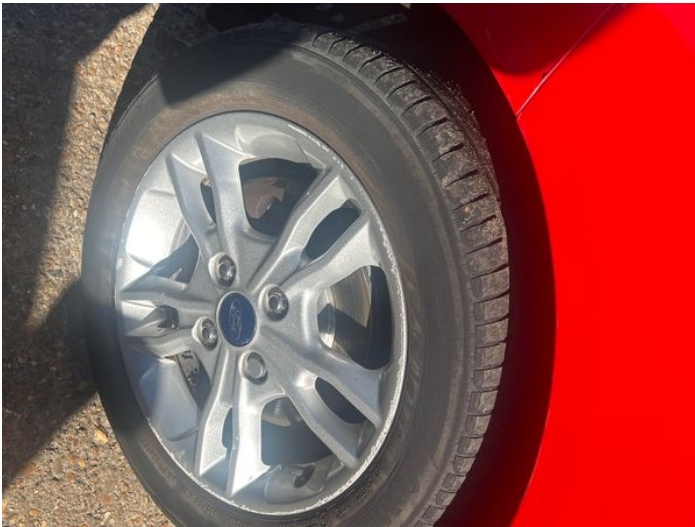
17: Wheel nsf Scratched Over 50mm
