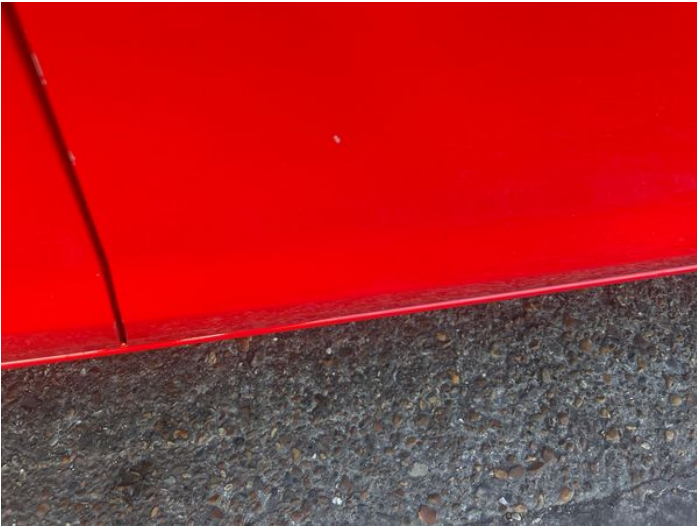
4: Door osf Chipped 1 To 5
