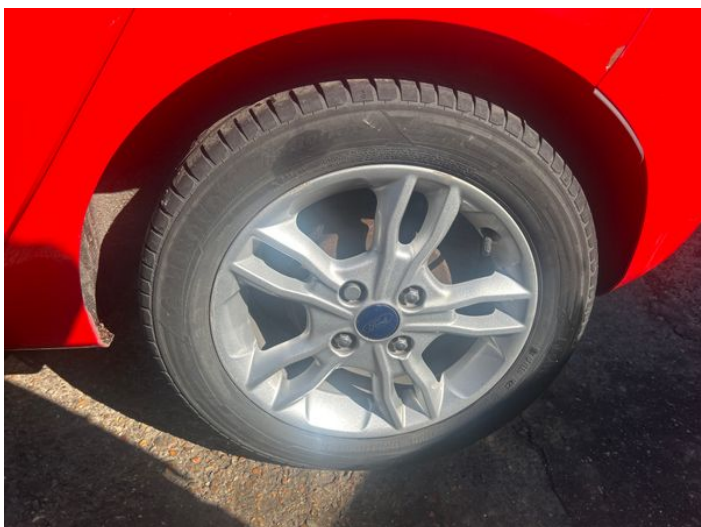
11: Wheel nsr Scratched Over 50mm
