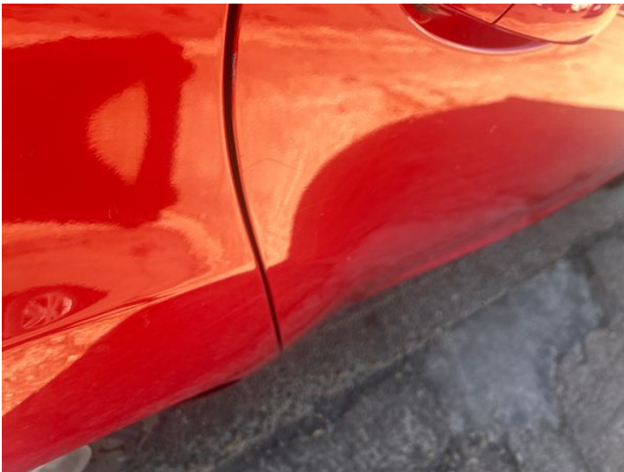
7: Door osr Chipped Edge Chip
