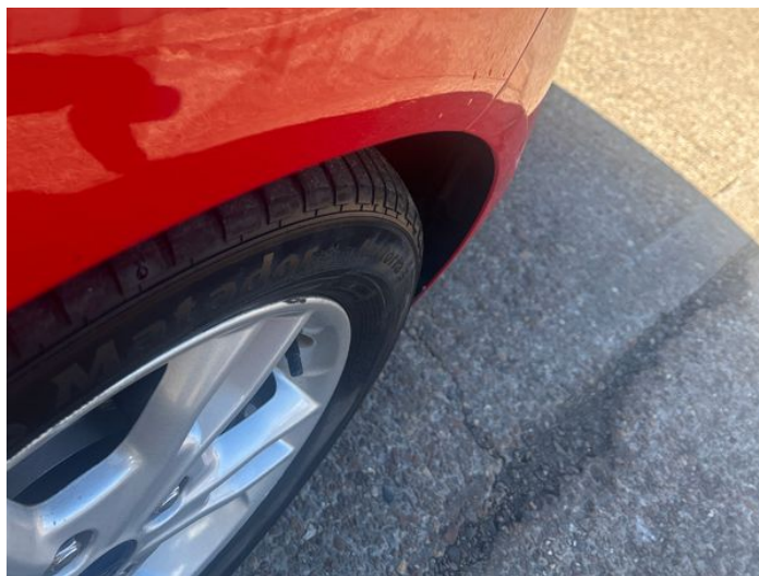
2: Wing osf Dented Between 10mm + 30mm
