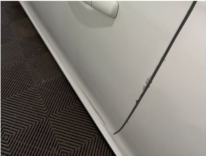
11: Door nsf Dented Over 30mm
