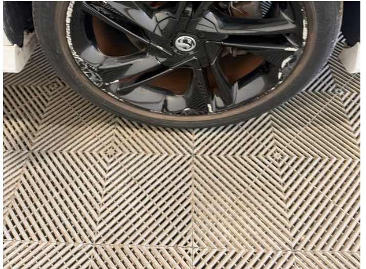
16: Wheel osf Scratched Over 50mm
