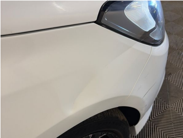
15: Wing osf Dented Over 30mm
