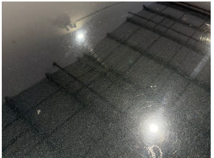
18: Roof Scratched Over 25mm Thru Paint
