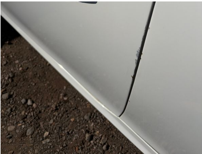
5: Door nsf Scratched Over 25mm Thru Paint
