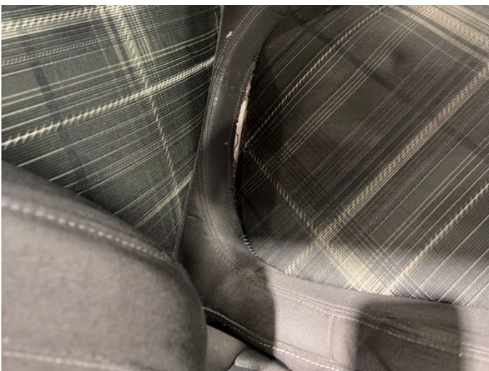
19: Seat Base Cover osf Torn Over 3mm
