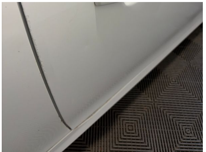
14: Door osf Dented With Paint Damage
