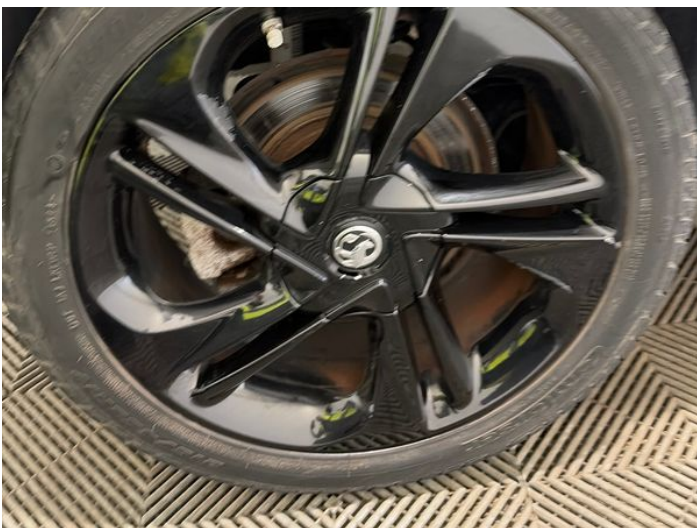
13: Wheel osr Scratched Up To 50mm
