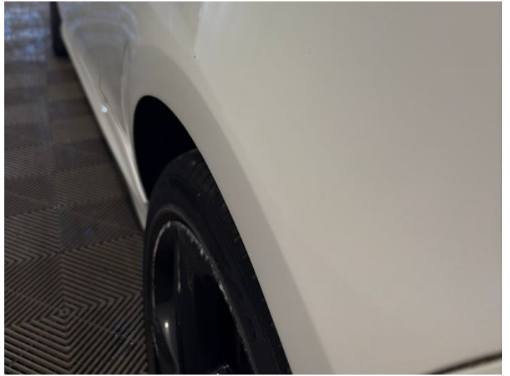
10: Qtr Panel nsr Poor Previous Repair Rippled UpTo 30%
