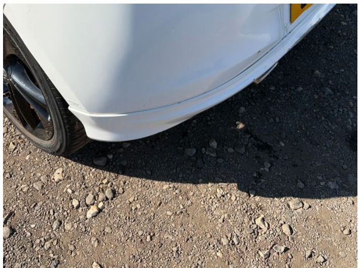
8: Bumper Rear Poor Previous Repair Poor Paint
