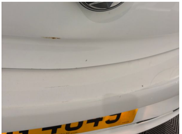
20: Tailgate Cracked Replace
