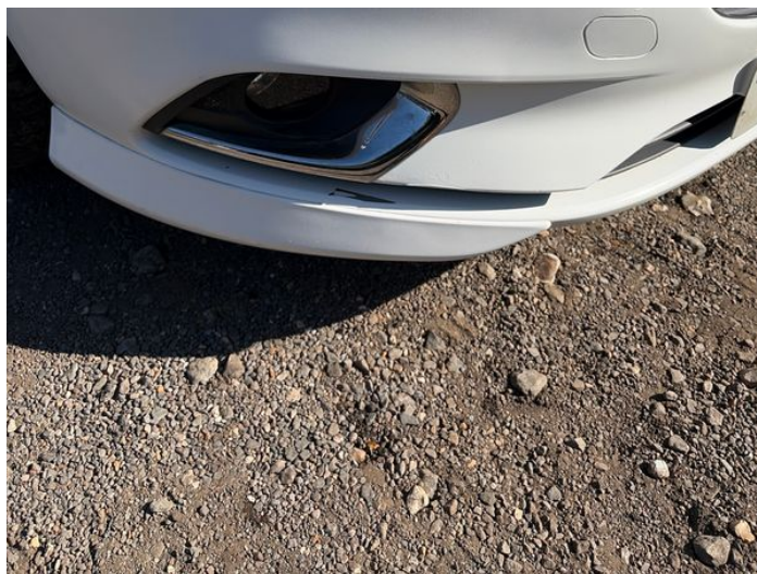
2: Bumper Front Poor Previous Repair Poor Paint
