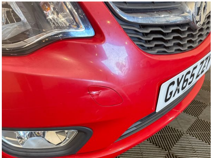
2: Bumper Front Dented With Paint Damage
