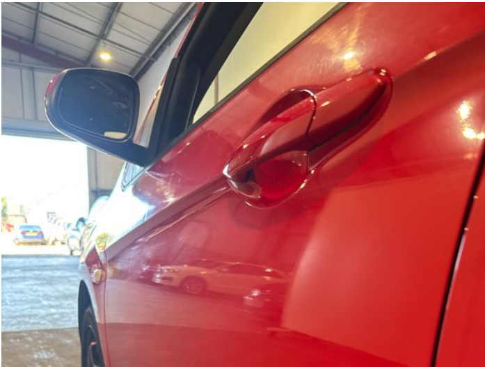
5: Door nsf Poor Previous Repair Rippled UpTo 30%
