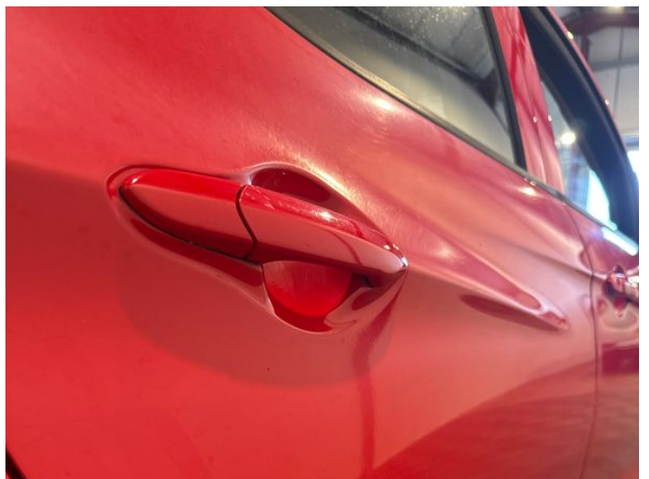
14: Door osr Poor Previous Repair Rippled UpTo 30%
