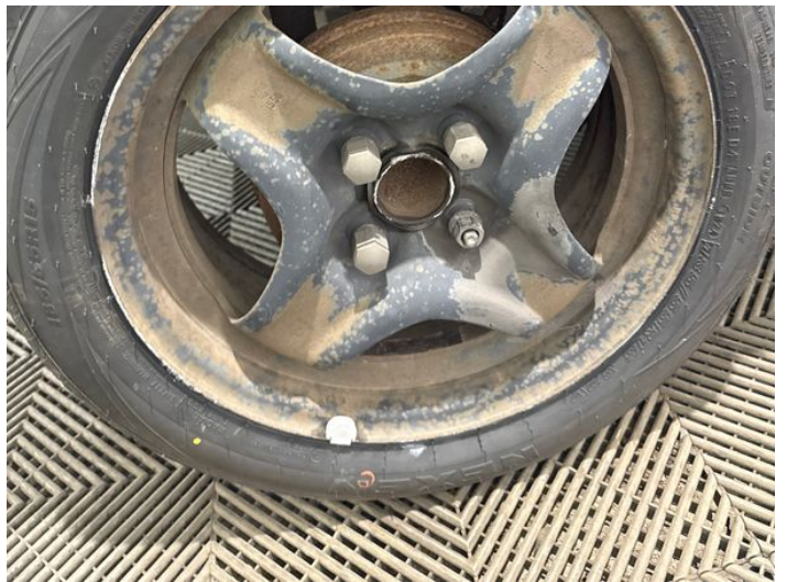
12: Wheel Trim osr Missing Replace
