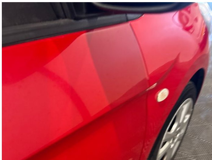
16: Door osf Dented With Paint Damage
