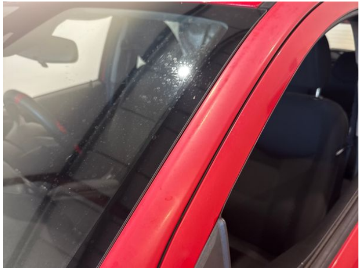
6: A Post ns Scratched Over 25mm Thru Paint
