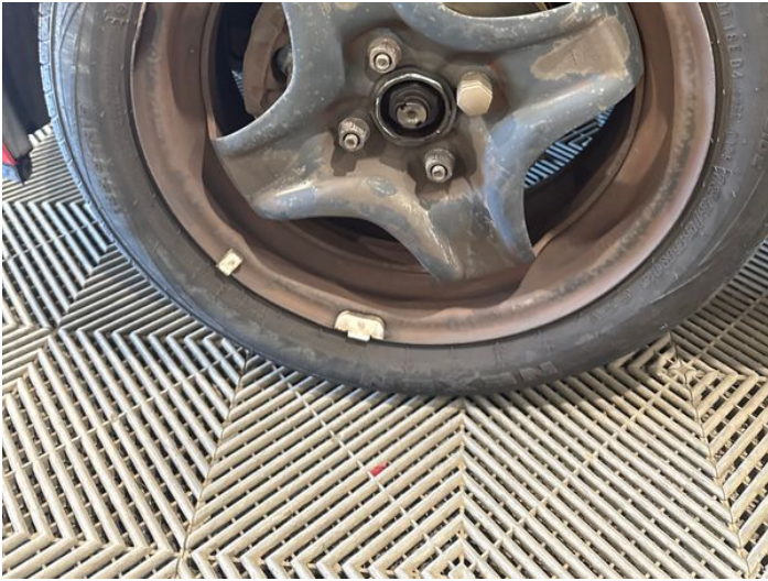
3: Wheel Trim nsf Broken Replace
