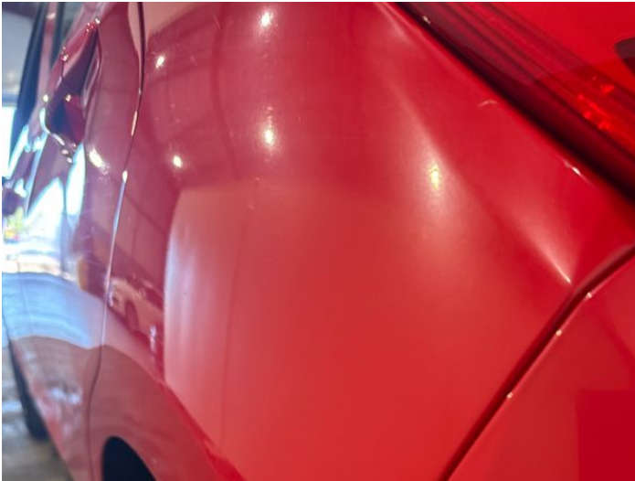
9: Qtr Panel nsr Dented Over 30mm
