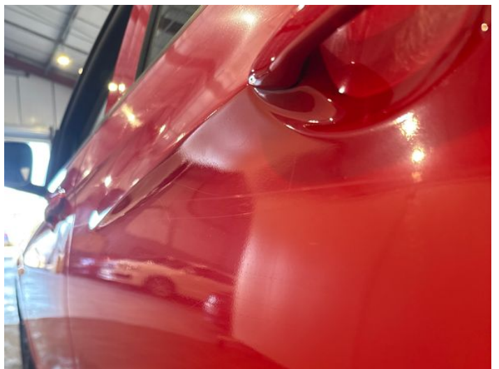
8: Door nsr Poor Previous Repair Rippled UpTo 30%
