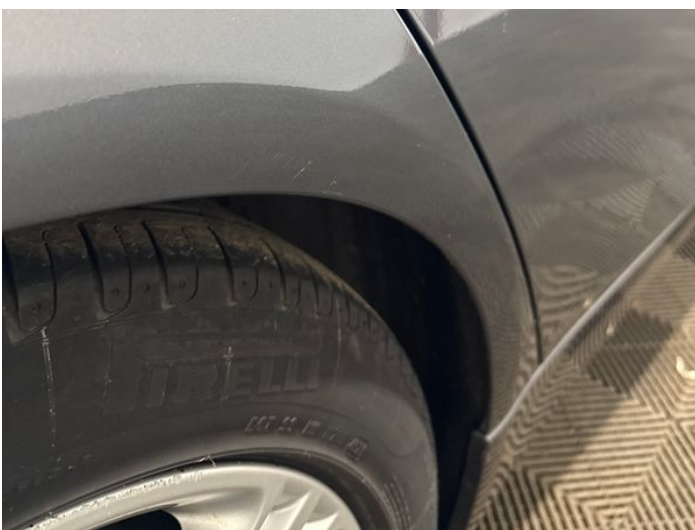
13: Qtr Panel osr Dented Between 10mm + 30mm
