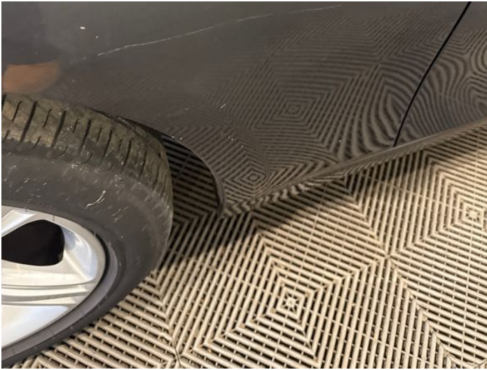
3: Wing nsf Scratched Over 25mm Thru Paint
