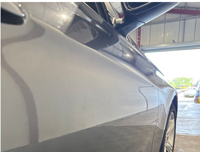
19: Door osf Dented Between 10mm + 30mm
