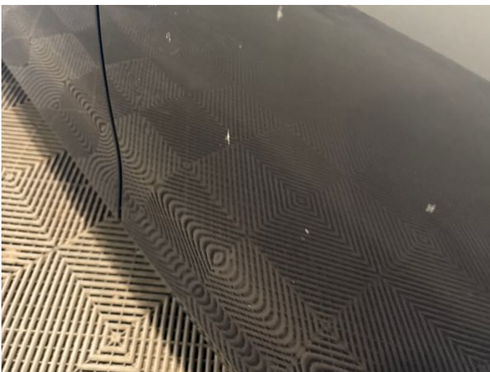
7: Door nsr Dented With Paint Damage
