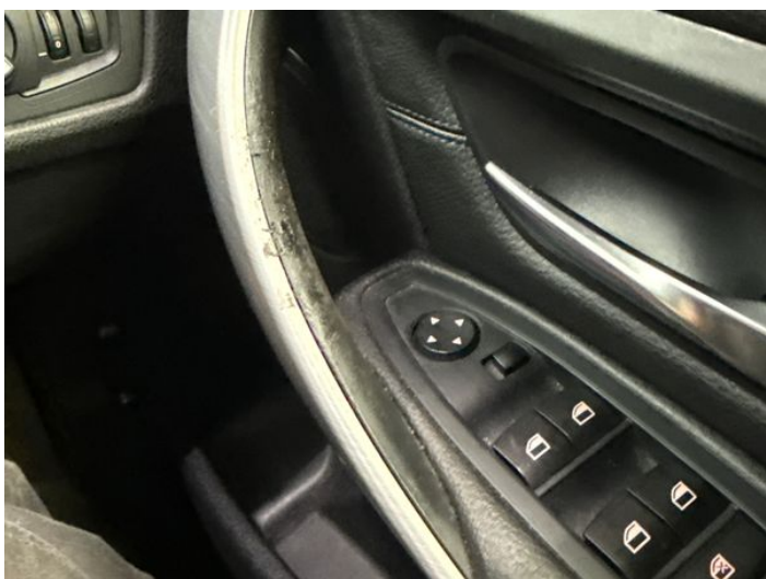
25: Door Pad osf Scuffed Over 25mm
