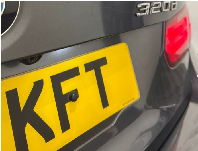
11: Boot Lid Scratched Over 25mm Thru Paint
