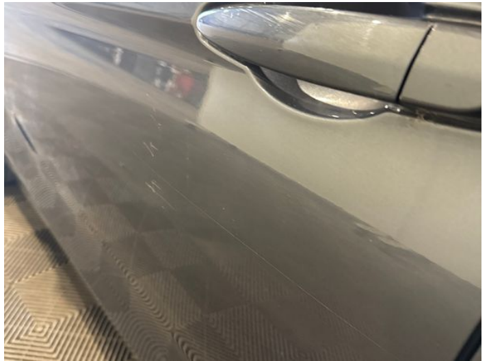
6: Door nsf Dented With Paint Damage
