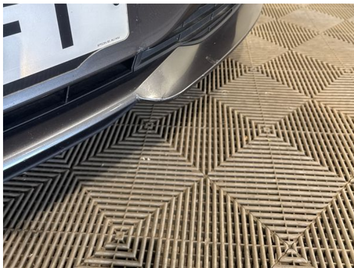
2: Bumper Front Dented With Paint Damage
