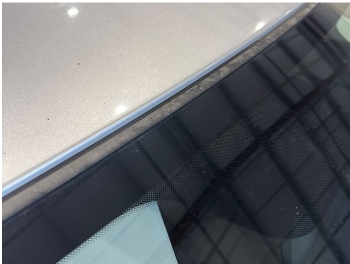
21: Roof Chipped Edge Chip
