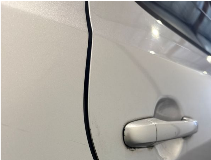
17: Door osr Scratched Over 25mm Thru Paint
