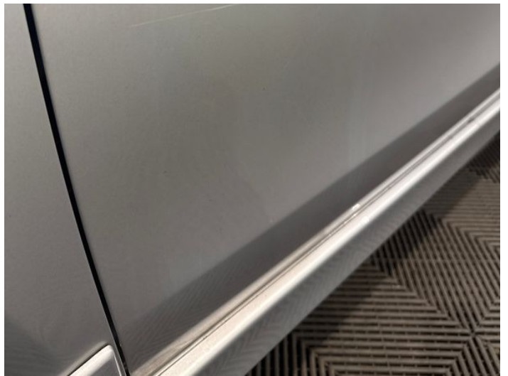
6: Door nsf Scratched Over 25mm Thru Paint
