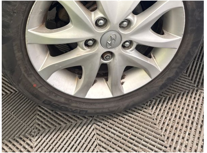
16: Wheel osr Scratched Over 50mm
