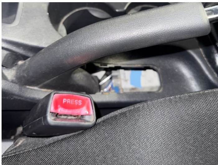
1: Fascia Trim Missing Replace
