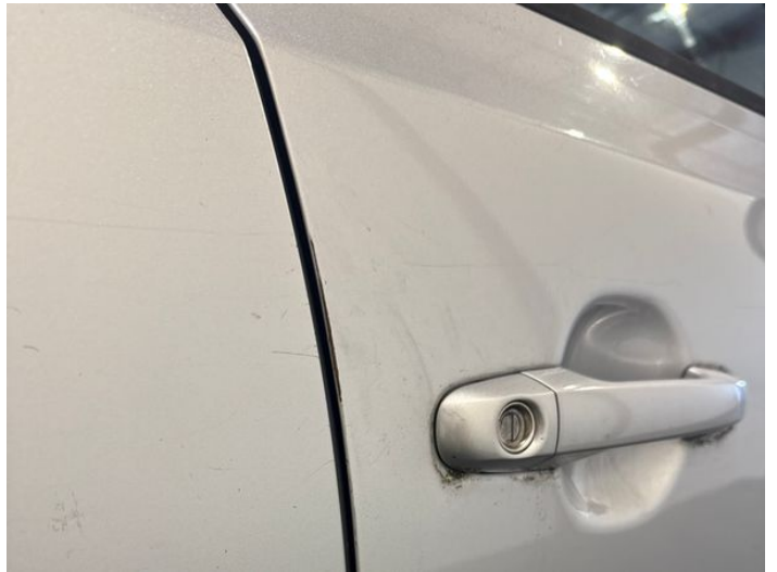
18: Door osf Scratched Over 25mm Thru Paint
