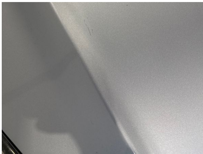
2: Bonnet Scratched Over 25mm Thru Paint
