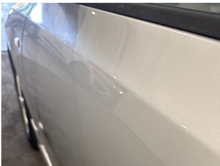
13: Door nsf Dented Over 30mm
