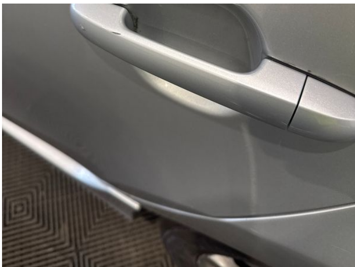
9: Door nsr Scratched UpTo 25mm Thru Paint
