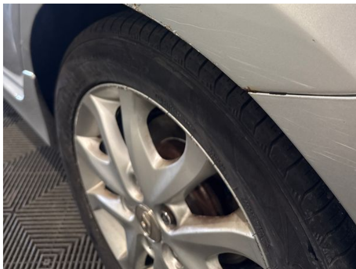
10: Qtr Panel nsr Scratched Rusted
