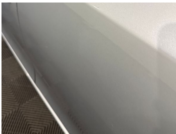
12: Door nsr Dented Between 10mm + 30mm
