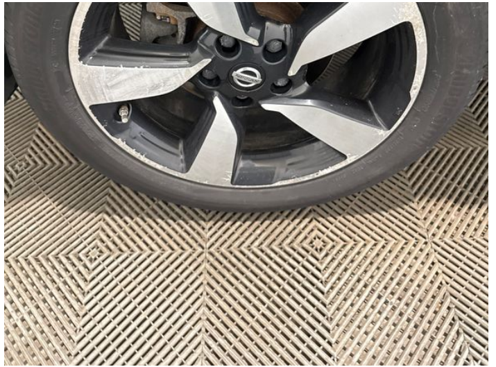
18: Wheel osr Scratched Over 50mm
