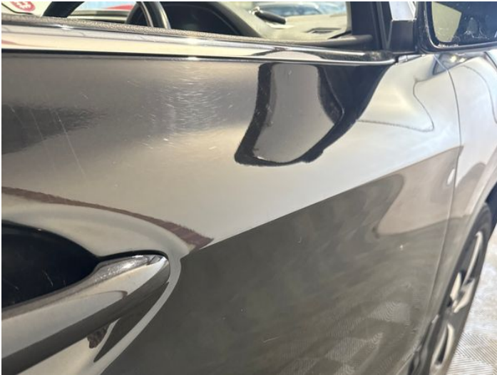
21: Door osf Scratched Over 25mm Thru Paint
