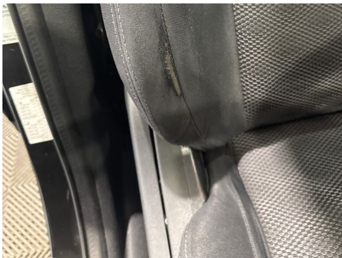
1: Seat Back Cover osf Scuffed Over 25mm
