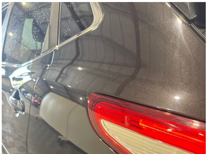
14: Qtr Panel nsr Poor Previous Repair Rippled UpTo 30%
