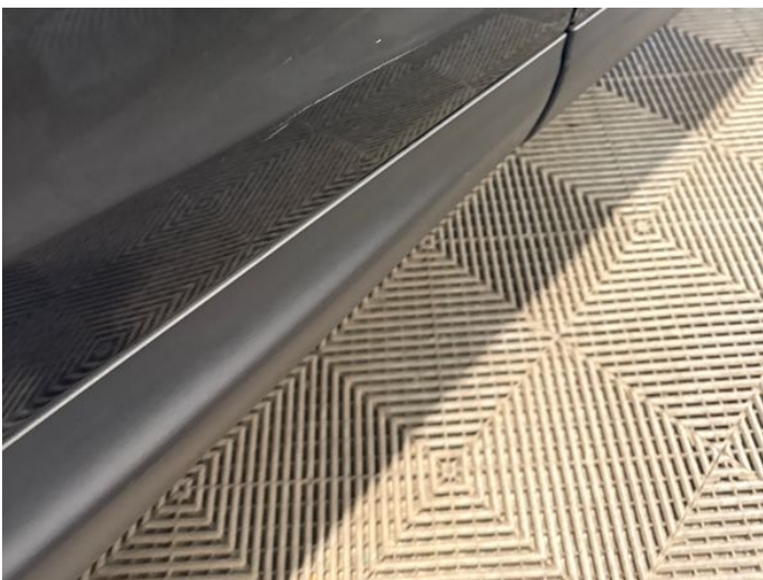
19: Door osr Scratched Over 25mm Thru Paint
