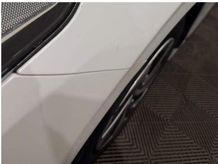
9: Wing nsf Chipped 1 To 5
