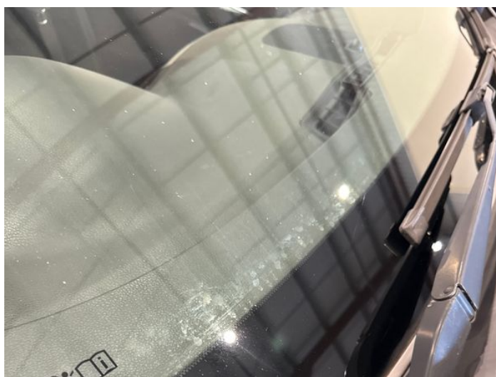
24: Screen Front Chipped UpTo 10mm
