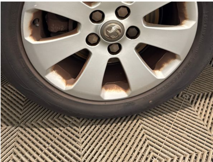
17: Wheel osr Scratched Over 50mm
