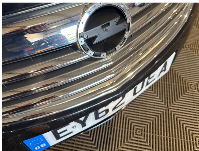
2: Badgedecal Front Missing Replace
