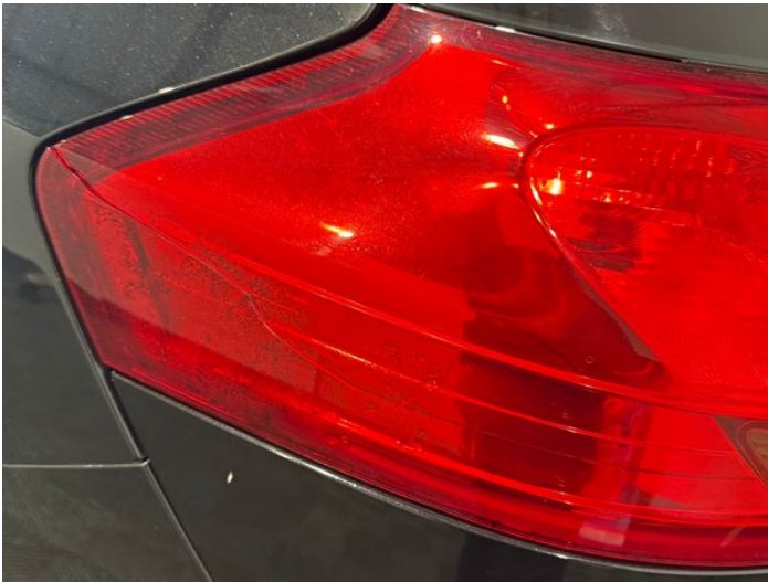
11: Lamp nsr Broken Replace
