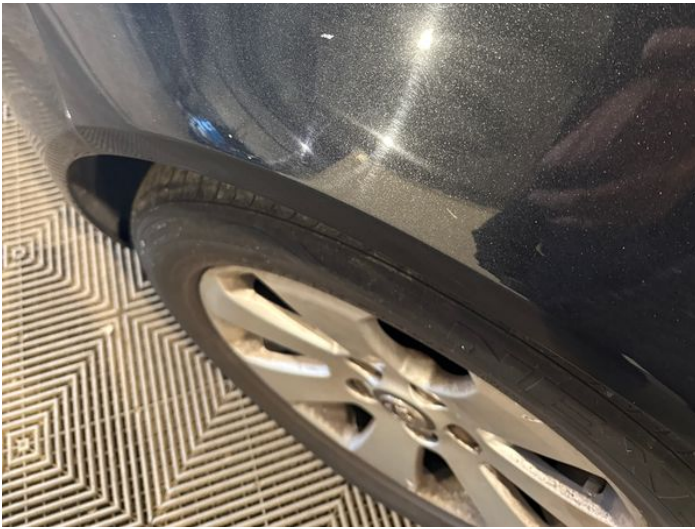
5: Wing nsf Scratched UpTo 25mm Thru Paint
