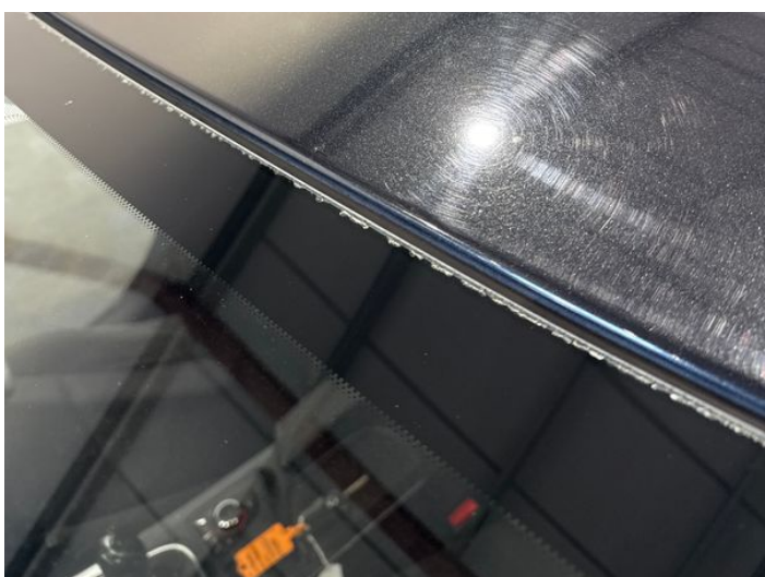
25: Roof Chipped Edge Chip
