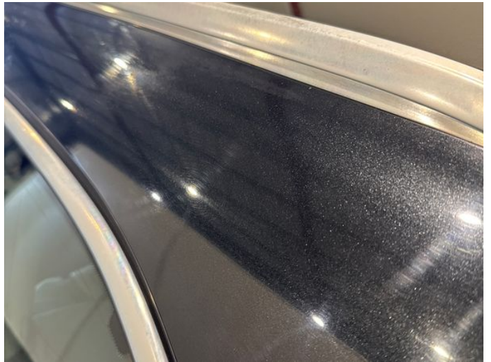
12: C Post ns Poor Previous Repair Poor Paint
