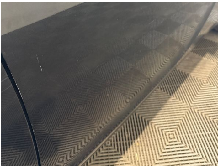
19: Door osf Scratched Over 25mm Thru Paint
