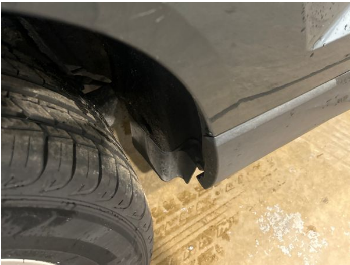
5: Door osr Scratched UpTo 25mm Thru Paint
