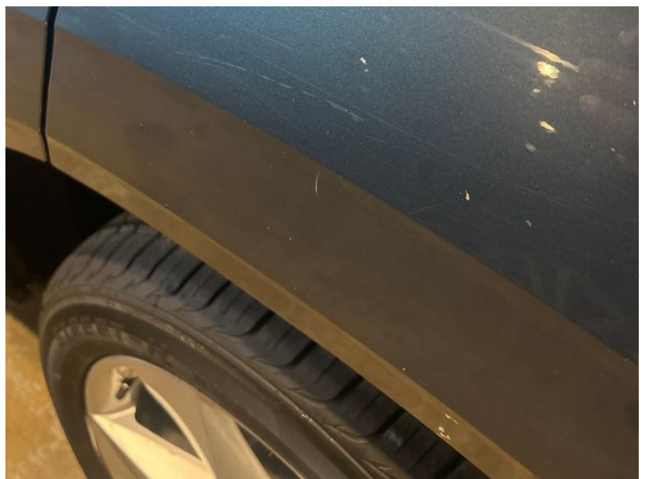
8: Qtr Panel nsr Chipped 1 To 5
