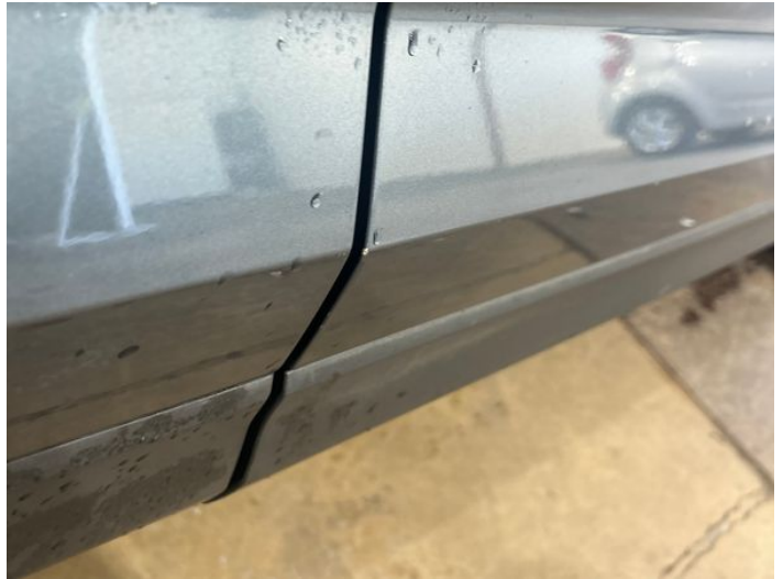
4: Door osf Chipped Edge Chip
