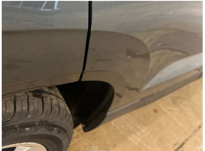
6: Door osr Chipped Edge Chip
