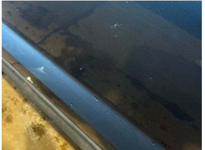
10: Door nsf Chipped 1 To 5
