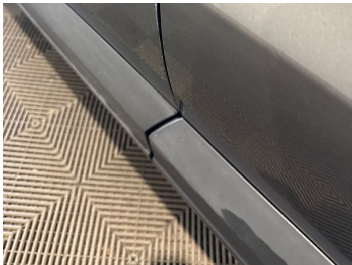
4: Door nsf Chipped Edge Chip
