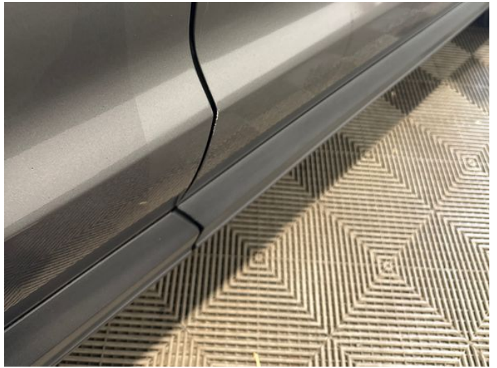
18: Door osf Chipped Edge Chip
