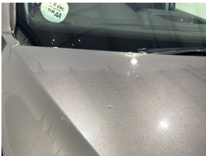
1: Bonnet Scratched Over 25mm Thru Paint
