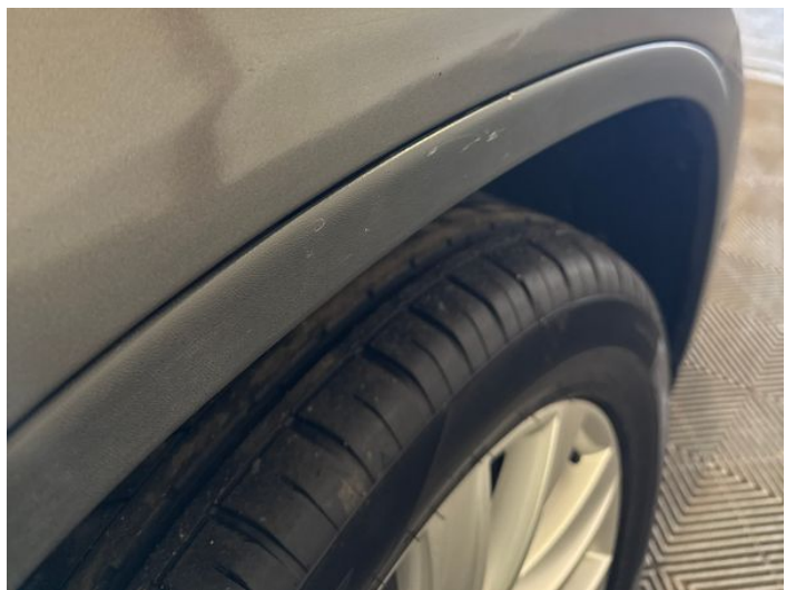
20: Wing osf Poor Previous Repair Rippled UpTo 30%
