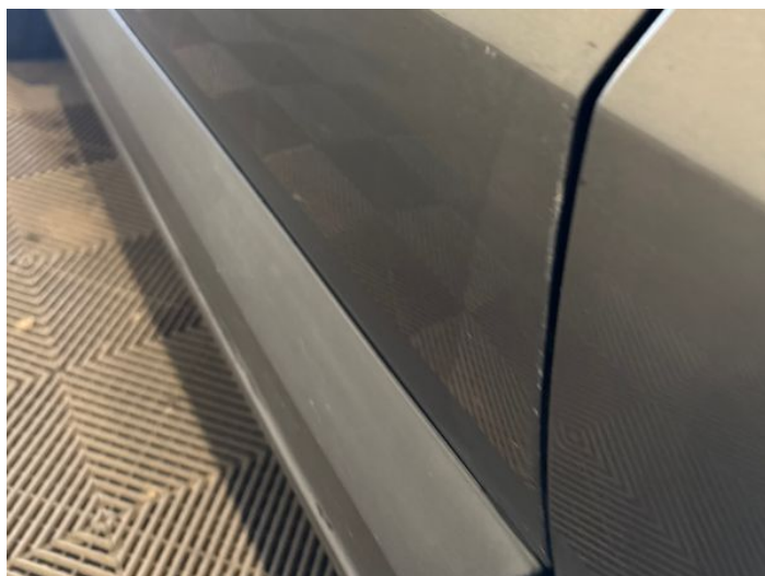
6: Door nsf Dented Between 10mm + 30mm
