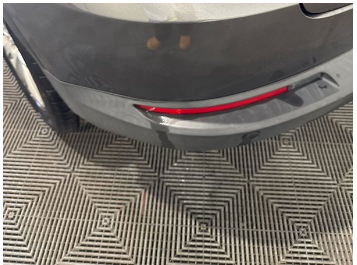
10: Bumper Rear Scratched 25 to 100mm Thru Paint
