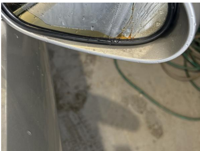
19: Door Mirror Glass os Broken Replace
