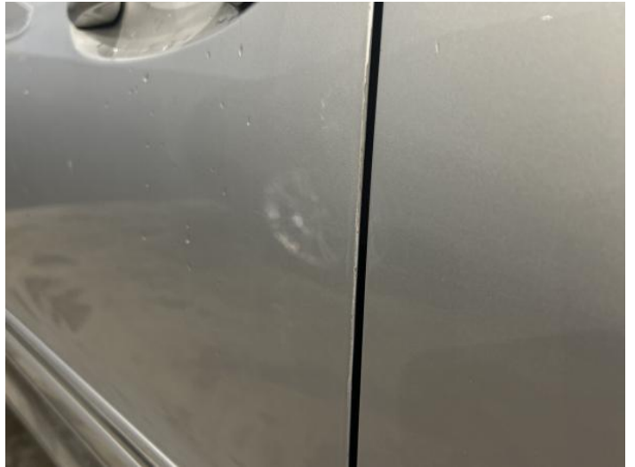
10: Door nsf Chipped Edge Chip
