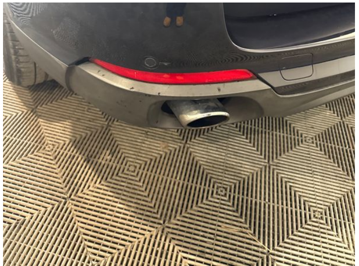
12: Bumper Rear Scratched 25 to 100mm Thru Paint
