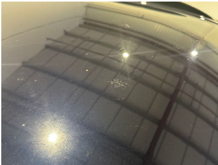
21: Roof Scratched Over 25mm Thru Paint
