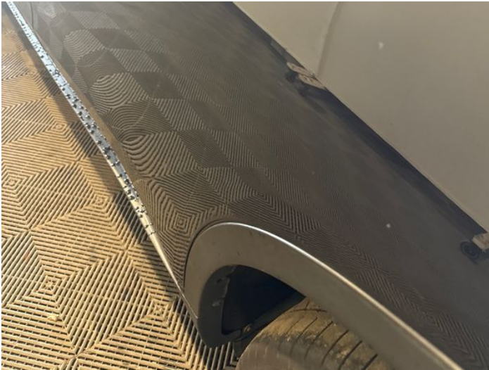
9: Door nsr Poor Previous Repair Rippled UpTo 30%
