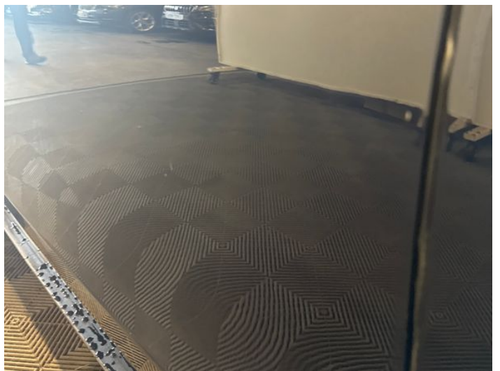
8: Door nsf Scratched UpTo 25mm Thru Paint
