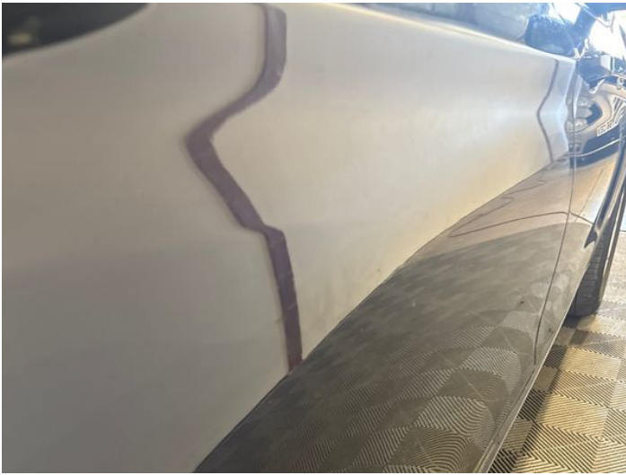
17: Door nsr Dented Between 10mm + 30mm
