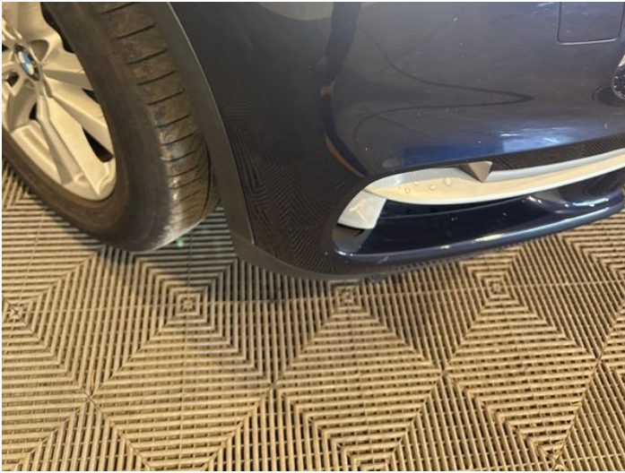
3: Bumper Front Scratched 25 to 100mm Thru Paint
