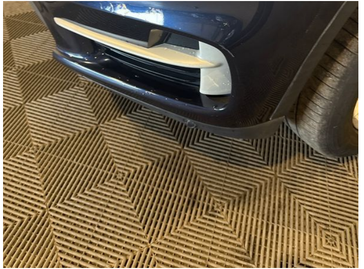
4: Bumper Front Scratched 25 to 100mm Thru Paint
