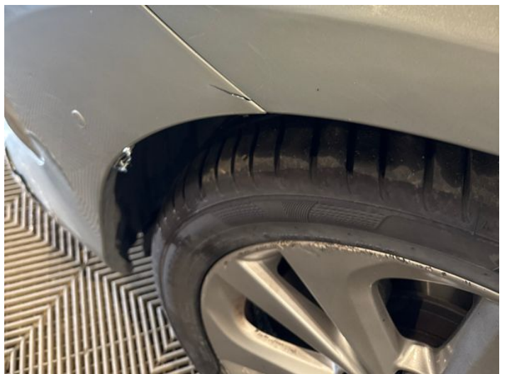
8: Wing nsf Scratched UpTo 25mm Thru Paint
