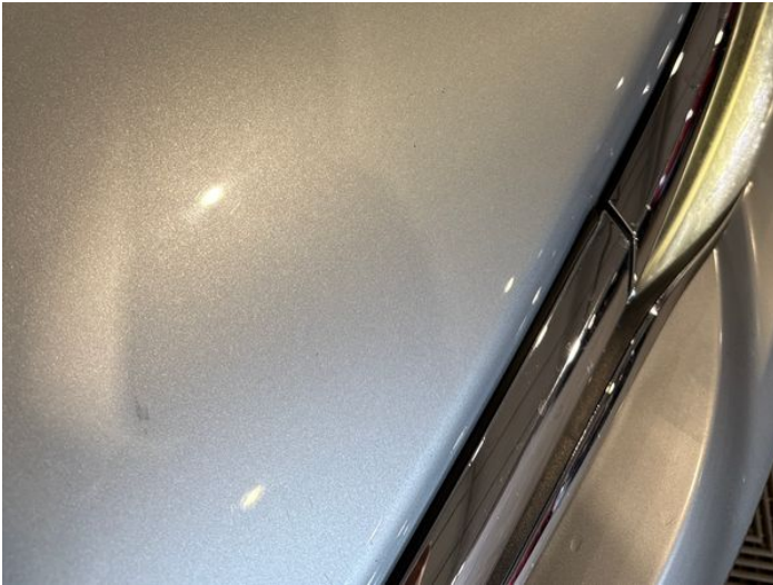
3: Bonnet Scratched Over 25mm Thru Paint
