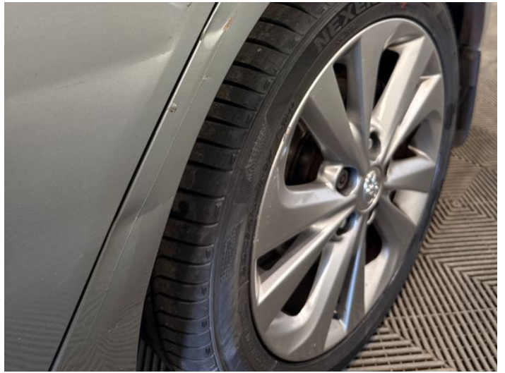
12: Qtr Panel nsr Dented With Paint Damage
