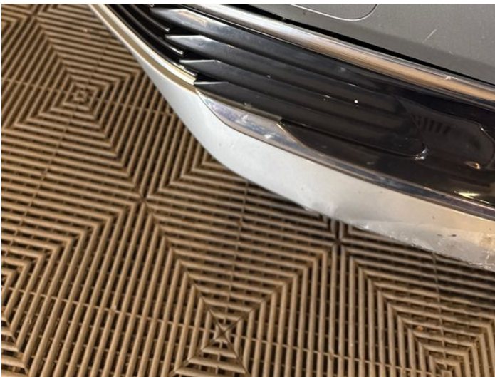
5: Bumper Front Moulding Broken Replace
