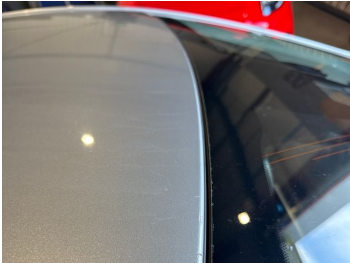
21: Roof Chipped Edge Chip
