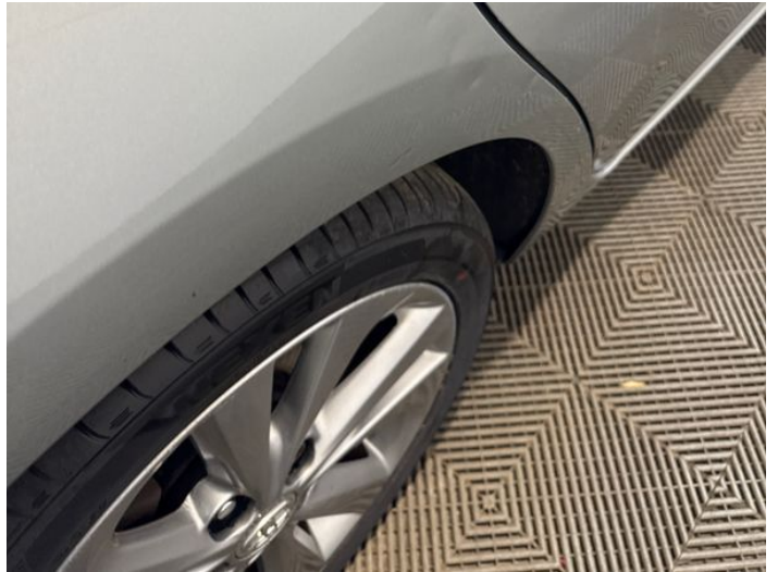
16: Qtr Panel osr Dented Over 30mm
