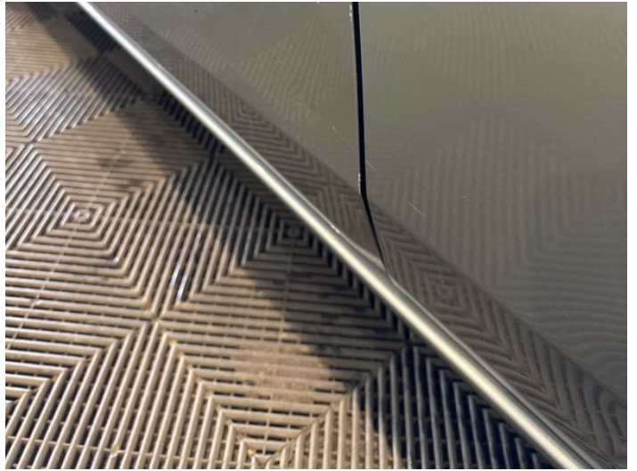
10: Door nsf Dented Between 10mm + 30mm
