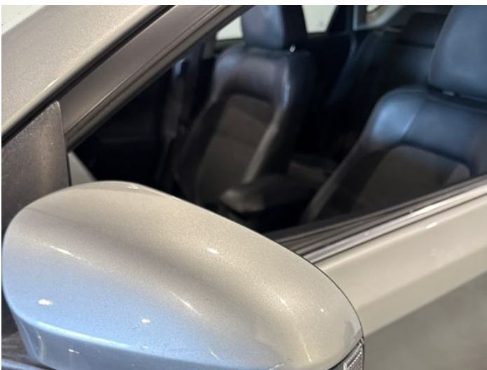
7: Door Mirror Assy nsf Scratched (Painted) UpTo 25mm Thru Paint
