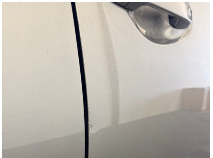
20: Door osf Chipped Edge Chip
