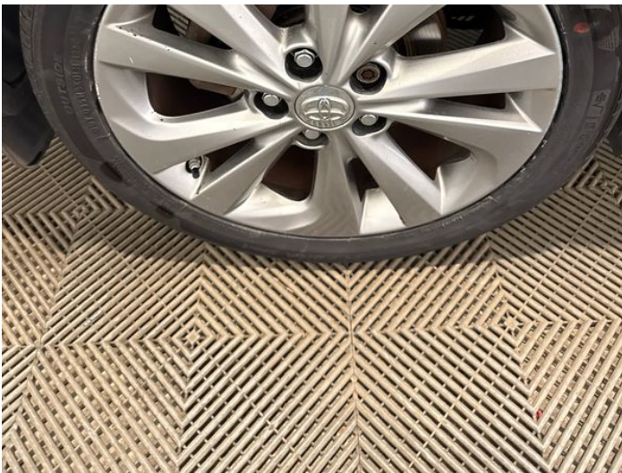
17: Wheel osr Scratched Over 50mm
