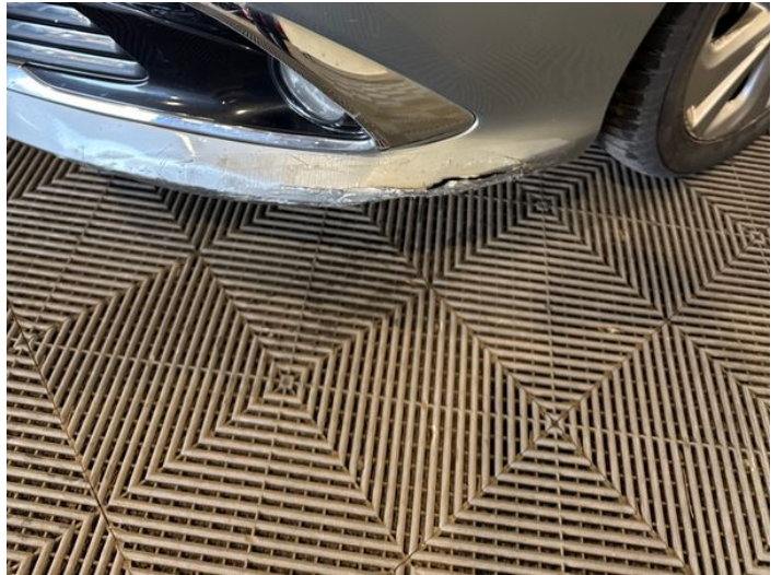
4: Bumper Front Cracked Over 25mm
