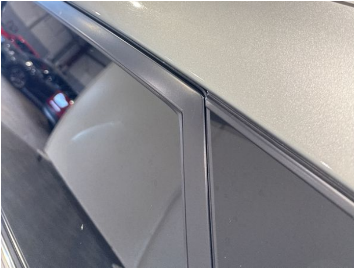
15: B Post ns Poor Previous Repair Poor Paint
