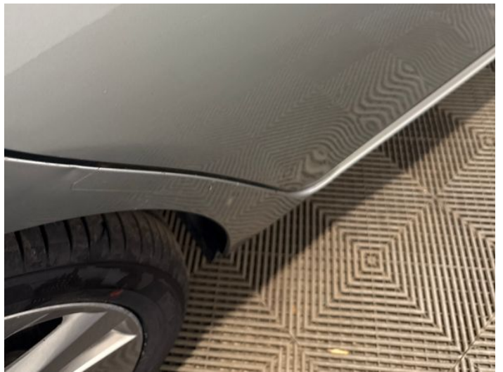
18: Door osr Scratched Over 25mm Thru Paint
