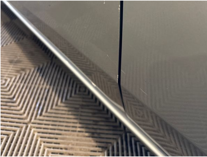
9: Door nsf Scratched Over 25mm Thru Paint
