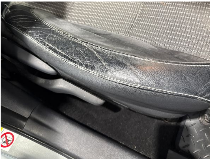
1: Seat Base Cover osf Scuffed Over 25mm
