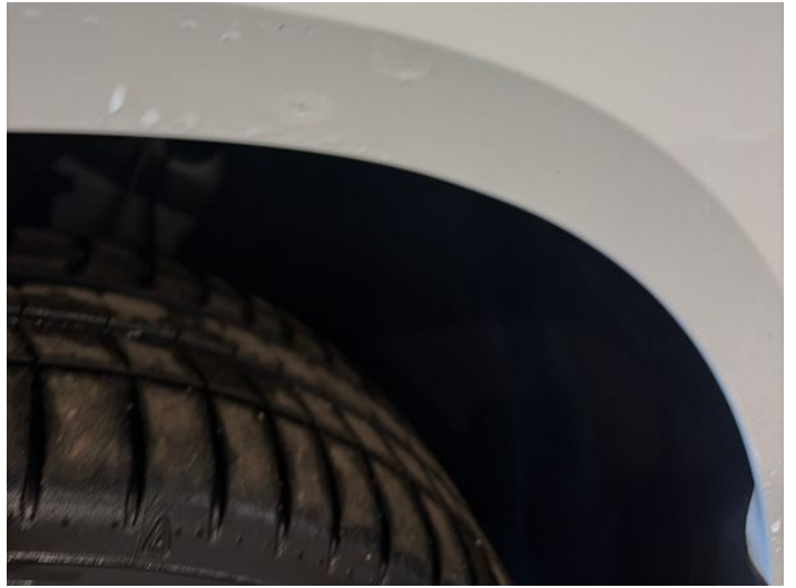
4: Wing nsf Scratched Over 25mm Thru Paint
