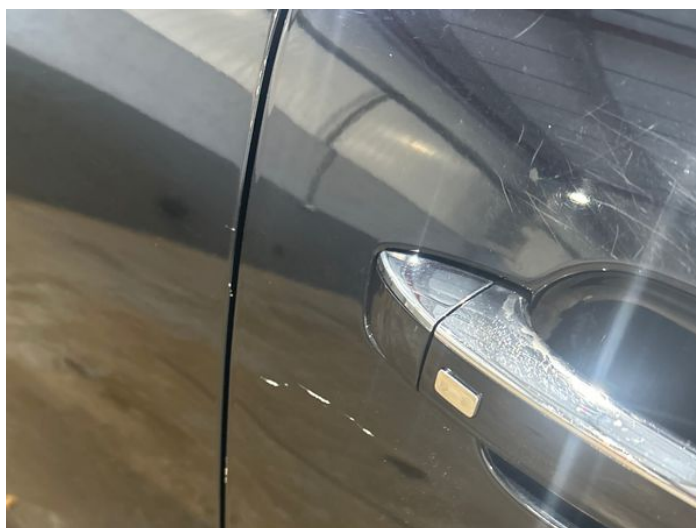
2: Door osf Scratched Over 25mm Thru Paint
