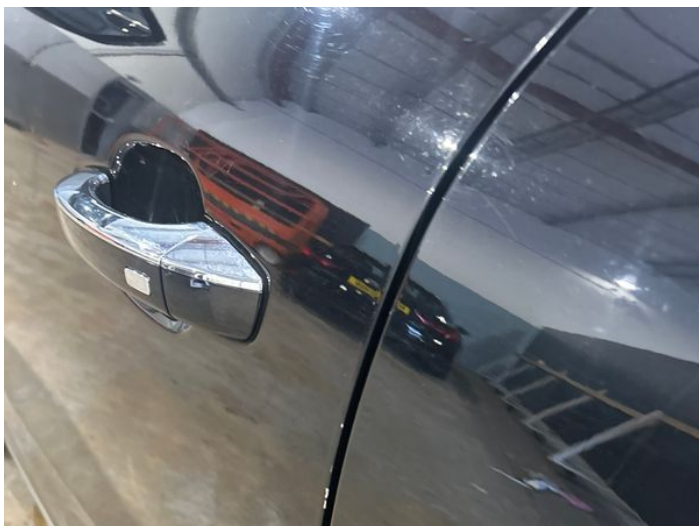
9: Door nsf Chipped Edge Chip
