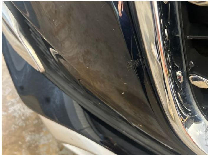
18: Bumper Front Chipped Multiple Chips
