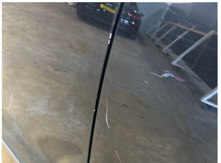
8: Door nsr Scratched Over 25mm Thru Paint
