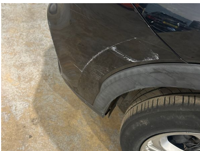
13: Bumper Front Scratched 25 to 100mm Thru Paint
