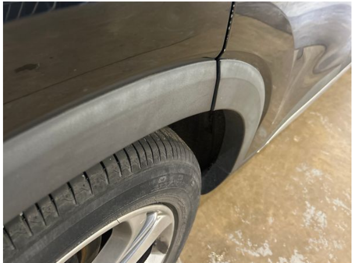
6: Qtr Panel osr Dented Between 10mm + 30mm
