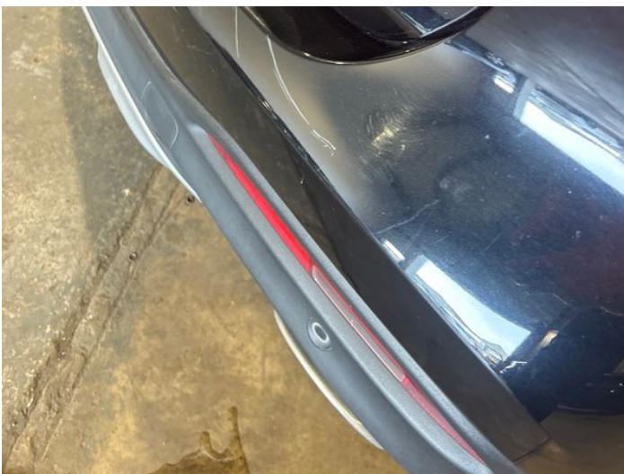
7: Bumper Rear Scratched 25 to 100mm Thru Paint
