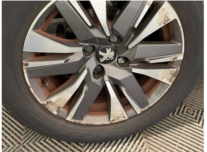
22: Wheel osr Scratched Over 50mm
