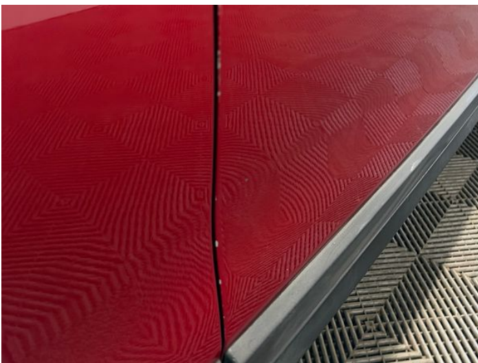
25: Door osf Chipped Edge Chip
