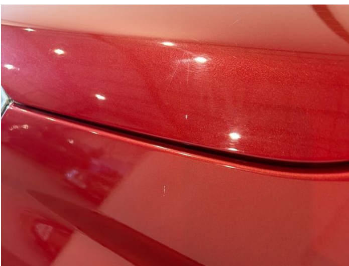
7: Wing nsf Scratched UpTo 25mm Thru Paint
