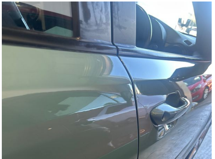
6: Door osr Dented Between 10mm + 30mm
