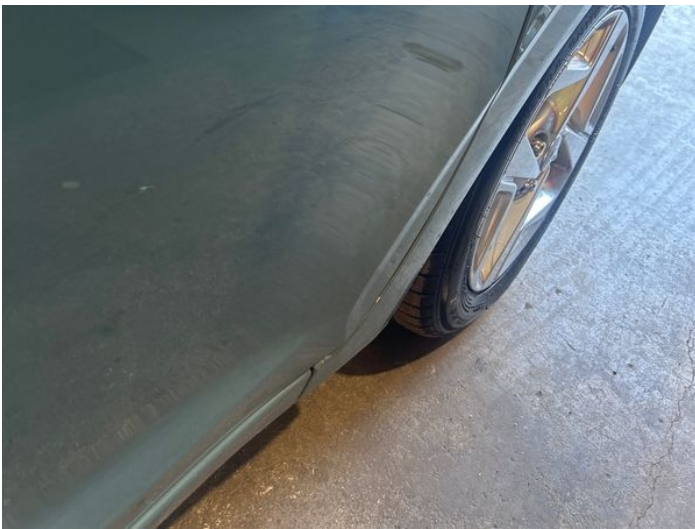
5: Door osf Dented Between 10mm + 30mm
