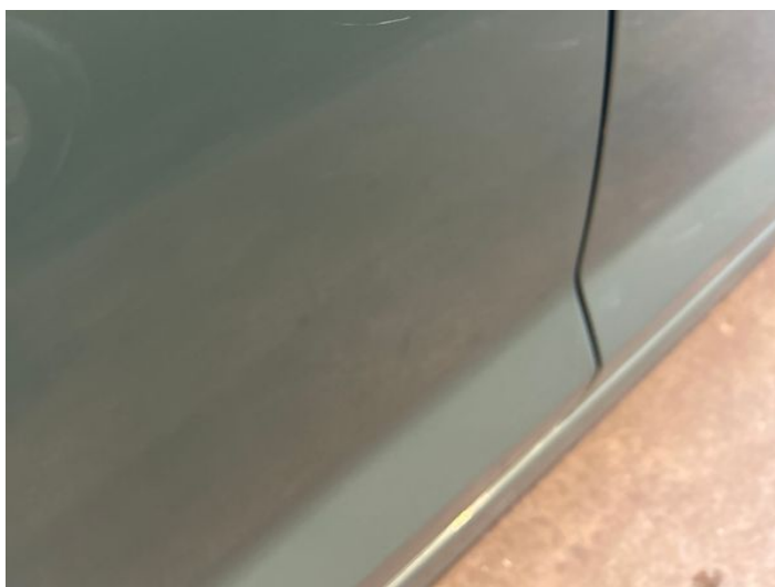
1: Door osr Scratched UpTo 25mm Thru Paint
