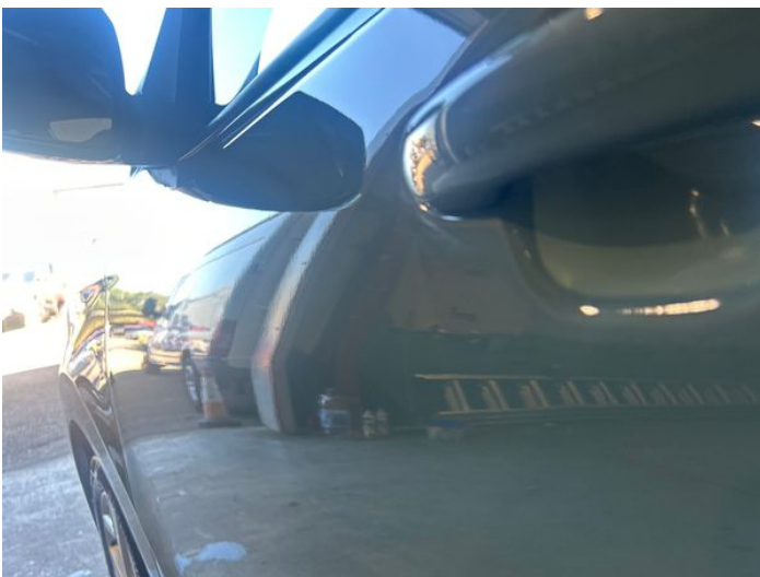
7: Door nsf Dented Between 10mm + 30mm
