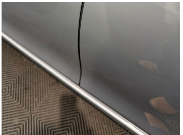
8: Door nsr Scratched Over 25mm Thru Paint
