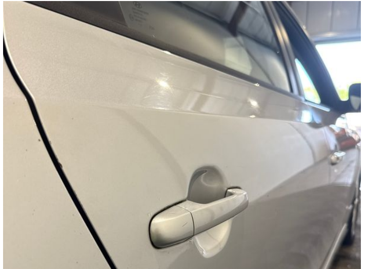
16: Door osr Poor Previous Repair Rippled UpTo 30%
