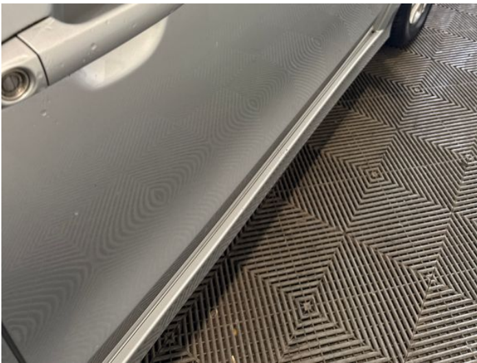
17: Door osf Dented With Paint Damage
