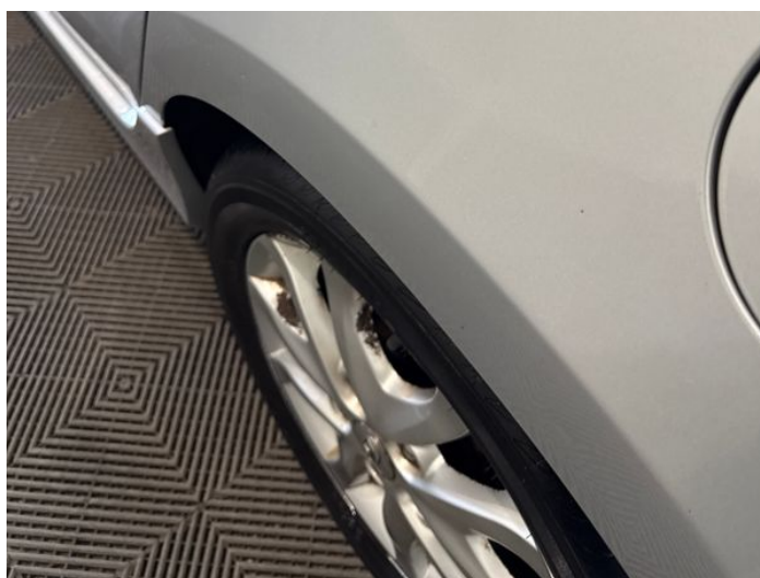
12: Qtr Panel nsr Dented Between 10mm + 30mm
