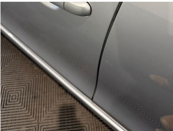
7: Door nsf Chipped Edge Chip
