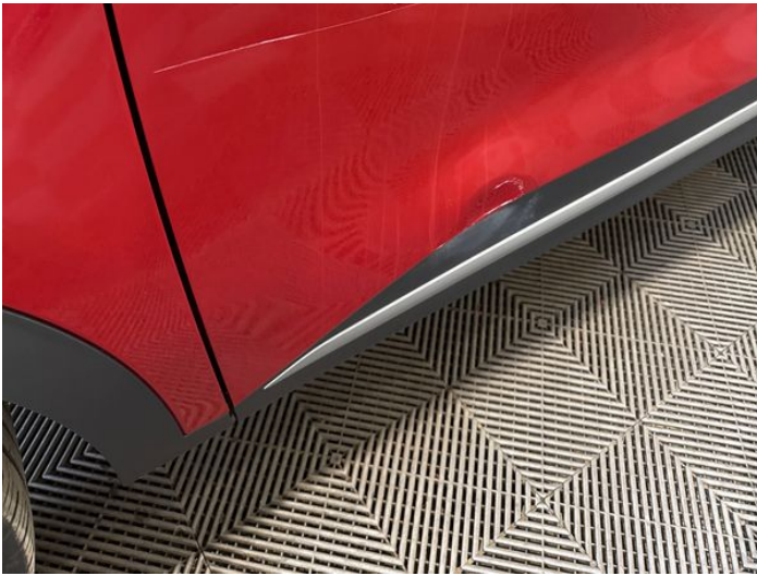
5: Door nsf Dented With Paint Damage
