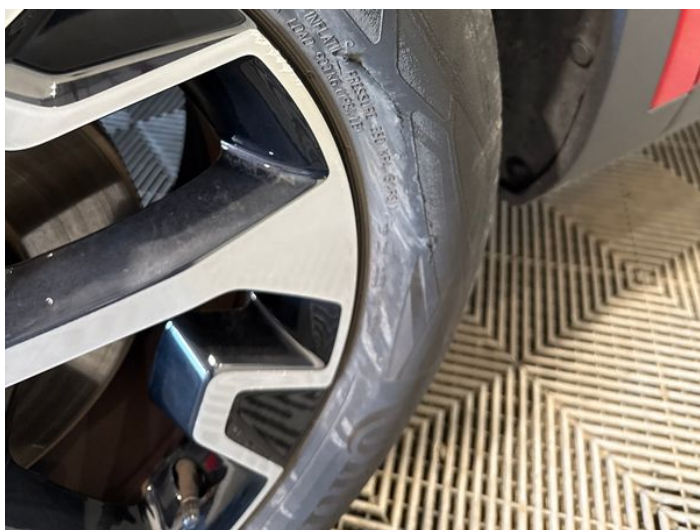
1: Tyre nsf Damaged Replace
