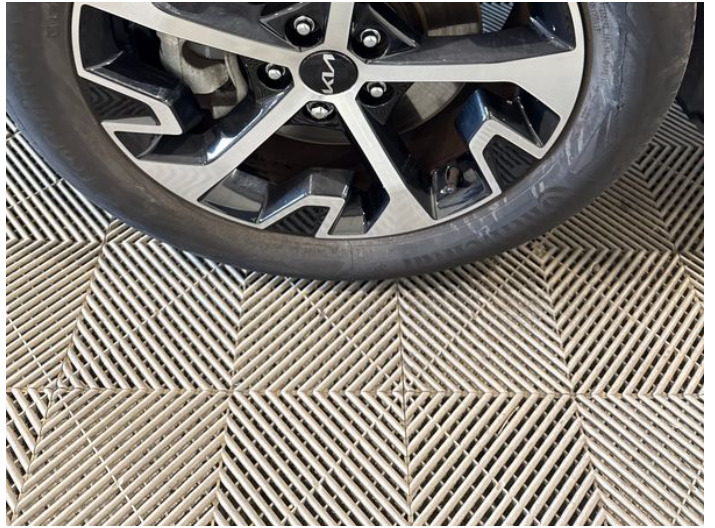
4: Wheel nsf Scratched Over 50mm
