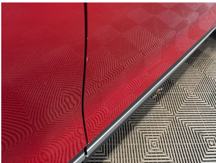
11: Door osf Chipped Edge Chip
