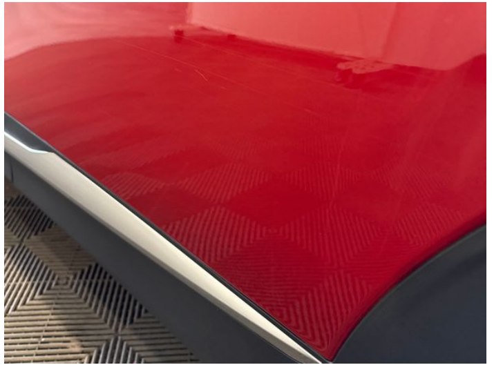
6: Door nsr Scratched UpTo 25mm Thru Paint
