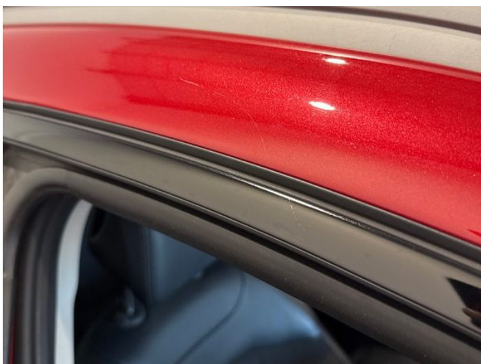
13: A Post os Scratched Over 25mm Thru Paint
