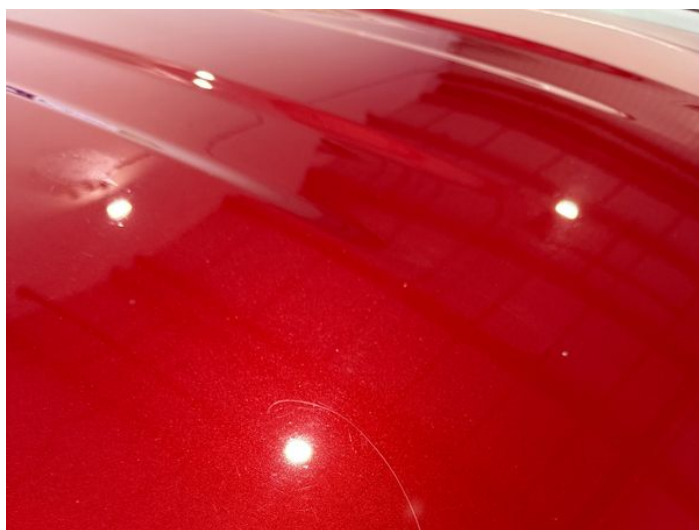
14: Roof Scratched Over 25mm Thru Paint
