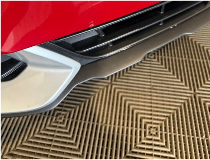
3: Bumper Front Scratched UpTo 25mm Thru Paint
