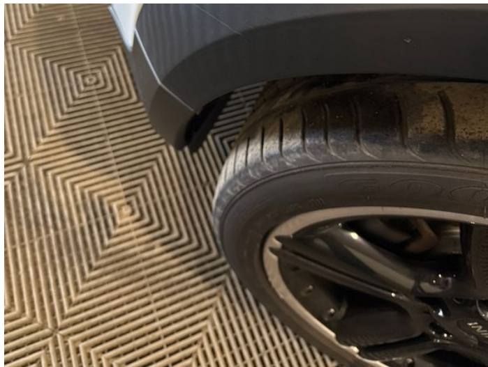
4: Wing Front Arch Extension ns Scuffed (Unpainted) UpTo 100mm
