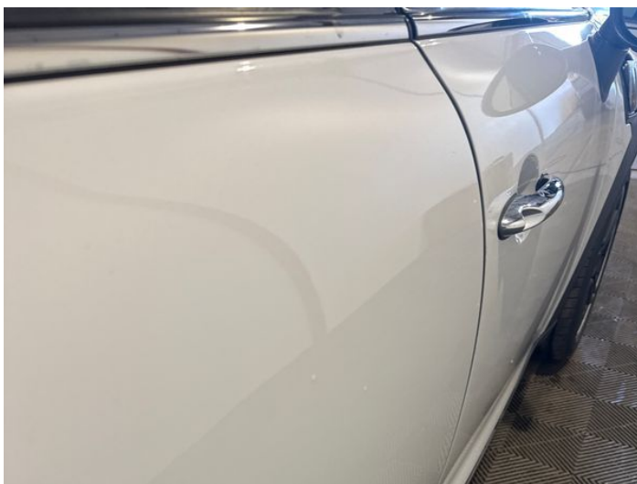
11: Door osr Dented Between 10mm + 30mm
