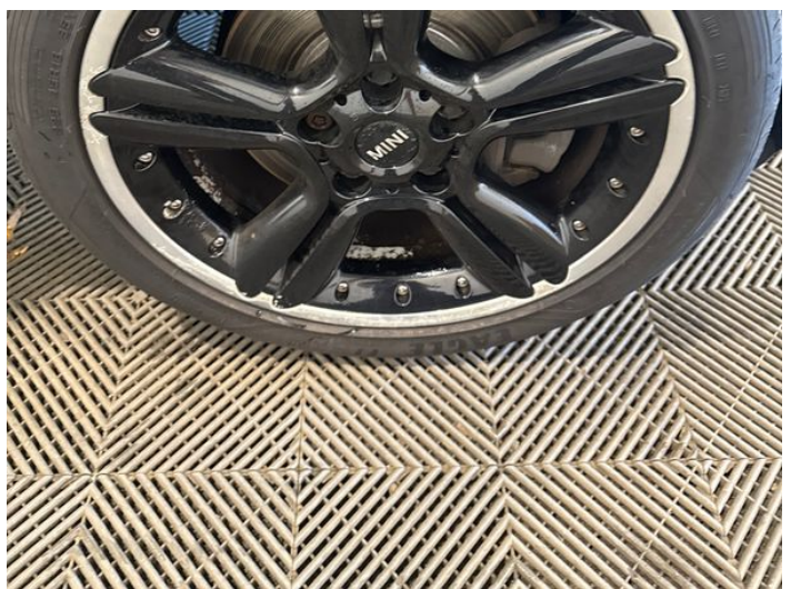
14: Wheel osf Scratched Over 50mm
