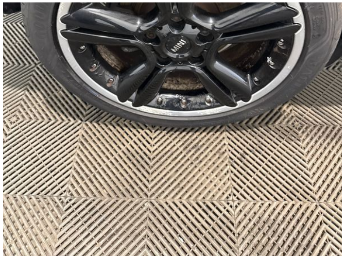
10: Wheel osr Scratched Over 50mm
