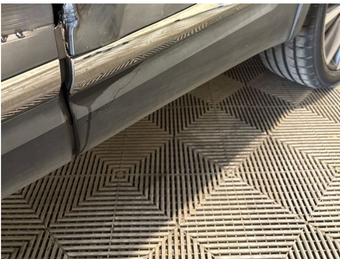
7: Door Moulding nsr Broken Replace
