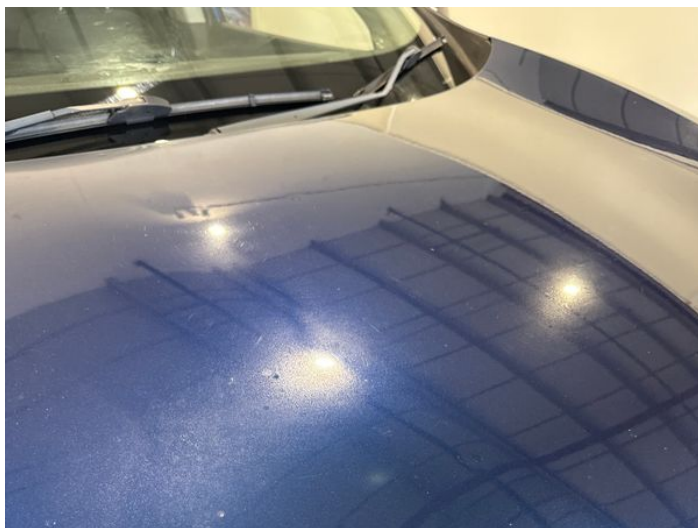
1: Bonnet Scratched Over 25mm Thru Paint
