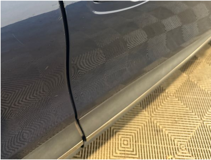
15: Door osf Chipped Edge Chip
