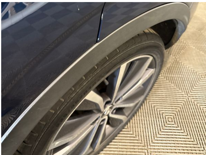
9: Qtr Panel nsr Chipped Edge Chip
