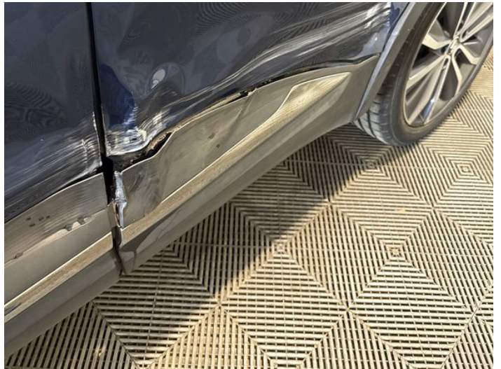
6: Door nsr Dented With Paint Damage
