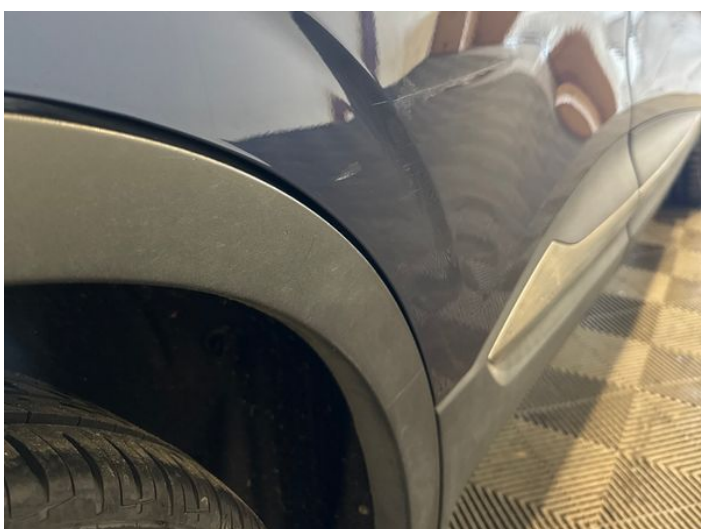
13: Door nsr Dented With Paint Damage
