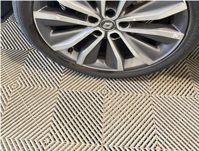
3: Wheel nsf Scratched Over 50mm
