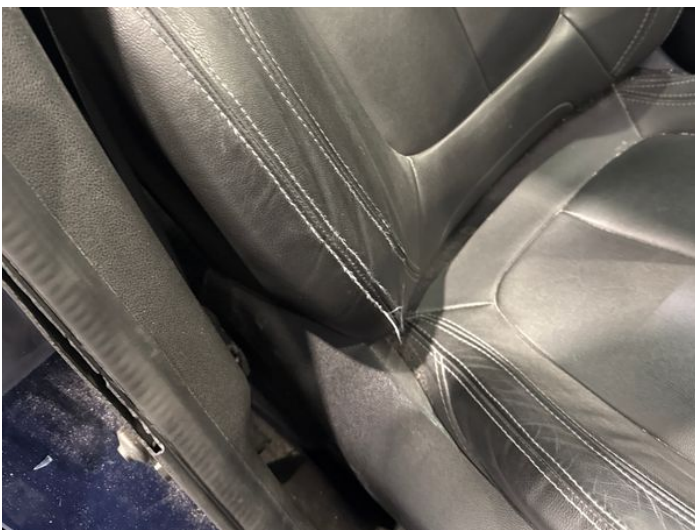
19: Seat Back Cover osf Scuffed Over 25mm
