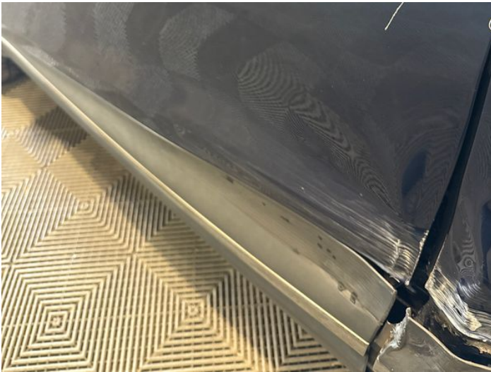
5: Door nsf Dented With Paint Damage
