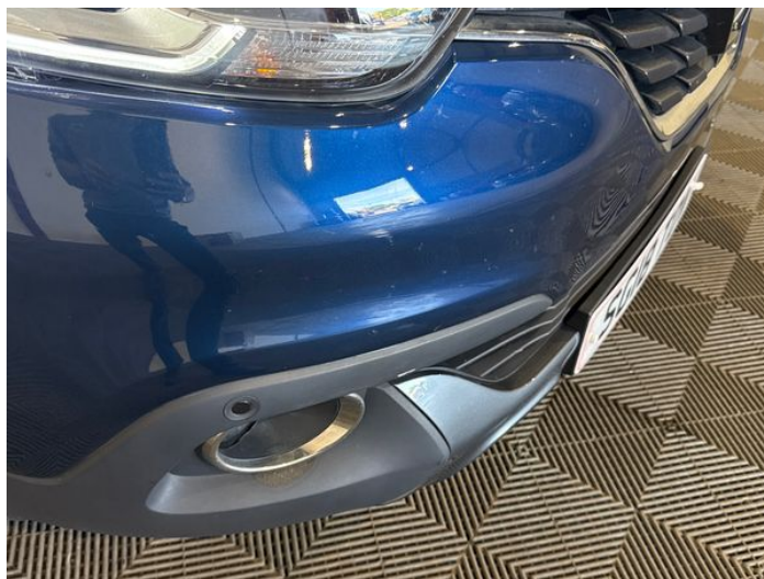
2: Bumper Front Scratched 25 to 100mm Thru Paint
