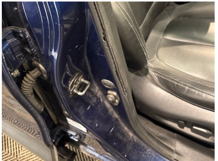
18: Aperture Seal osf Broken Replace
