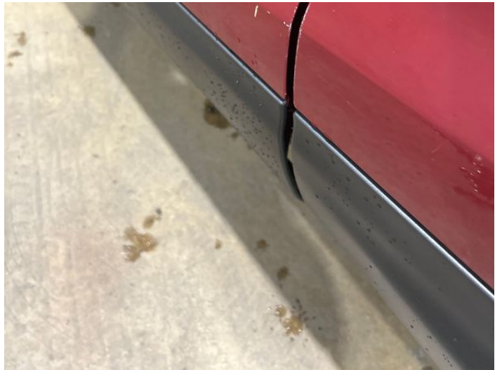
12: Door nsf Chipped Edge Chip
