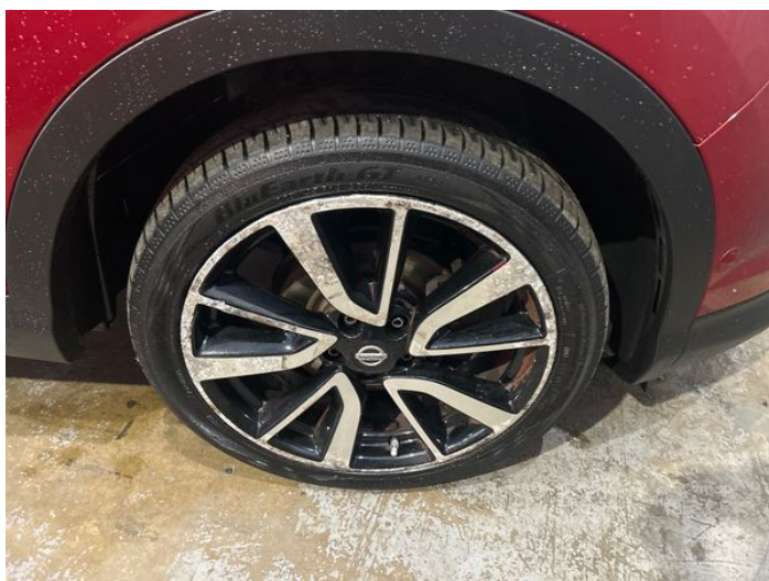
1: Wheel osf Corroded Light
