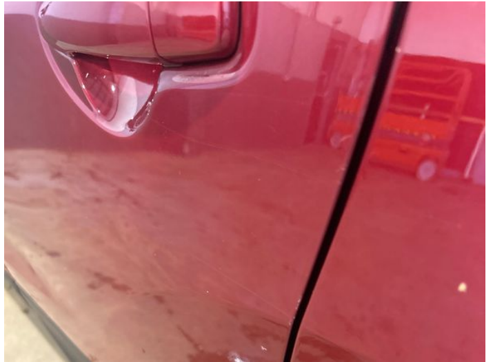
10: Door nsr Chipped Edge Chip
