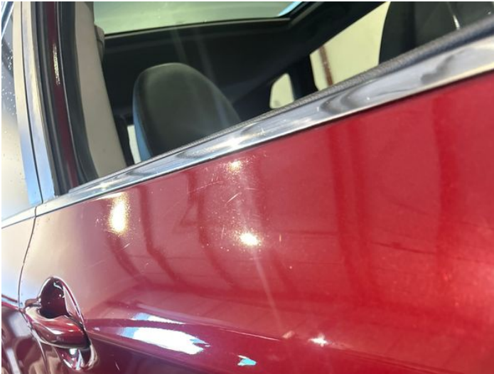
3: Door osf Dented Over 30mm
