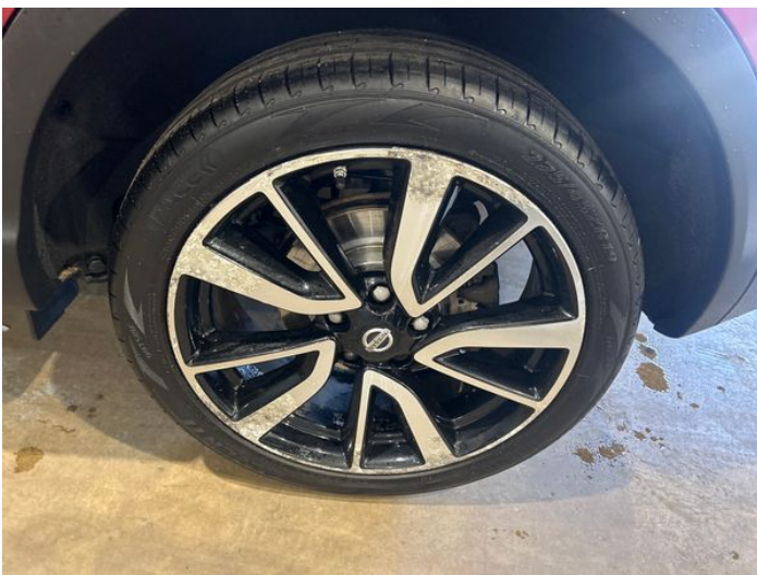
7: Wheel nsr Corroded Light
