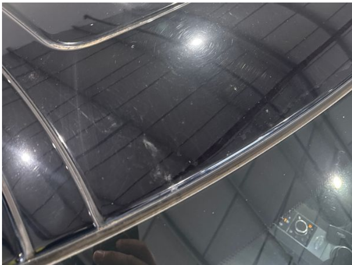
17: Roof Scratched Over 25mm Thru Paint
