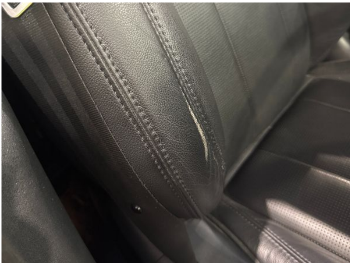
18: Seat Back Cover osf Scuffed Over 25mm
