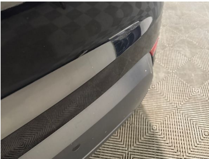
11: Tailgate Poor Previous Repair Poor Paint
