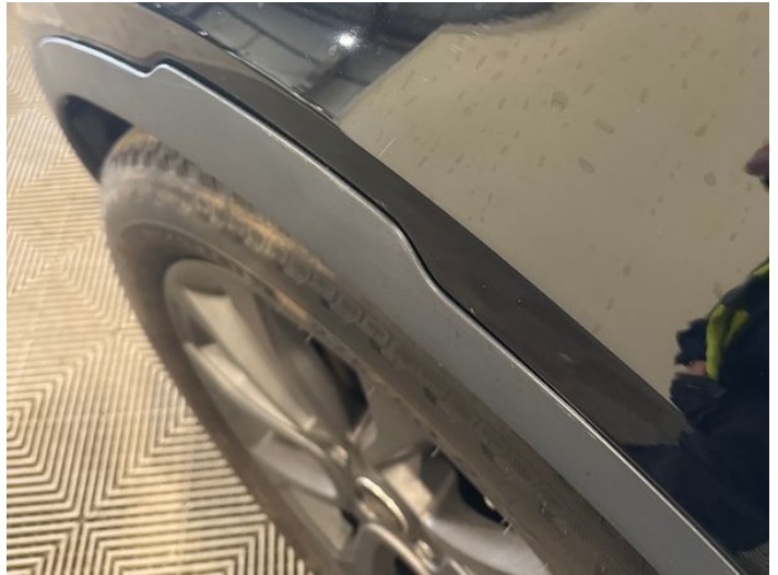
4: Wing nsf Scratched UpTo 25mm Thru Paint
