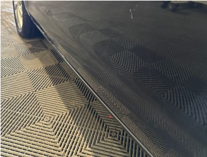
9: Door nsf Dented Between 10mm + 30mm
