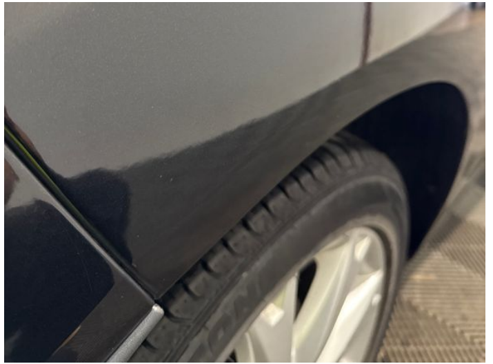
18: Qtr Panel osr Poor Previous Repair Poor Paint
