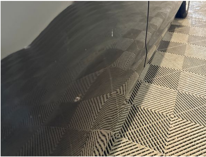
17: Qtr Panel osr Dented Between 10mm + 30mm
