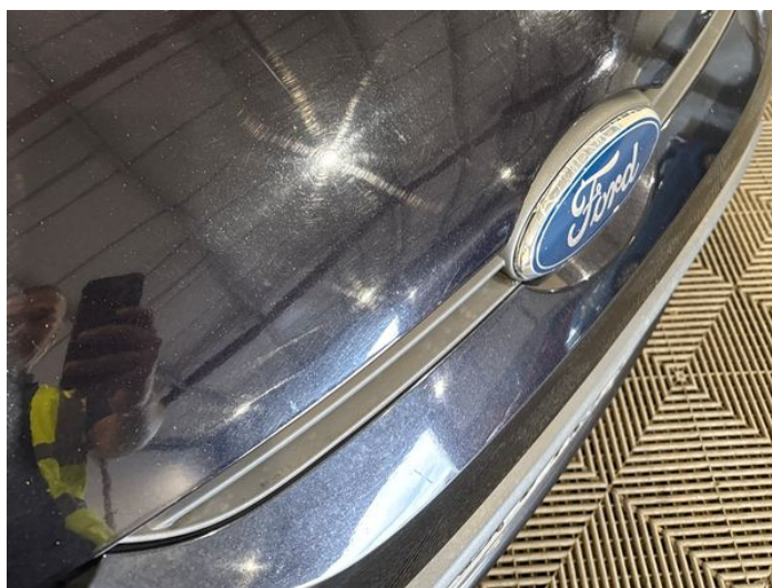
2: Bonnet Scratched Over 25mm Thru Paint
