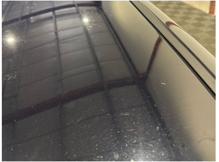
16: Roof Dented Over 30mm
