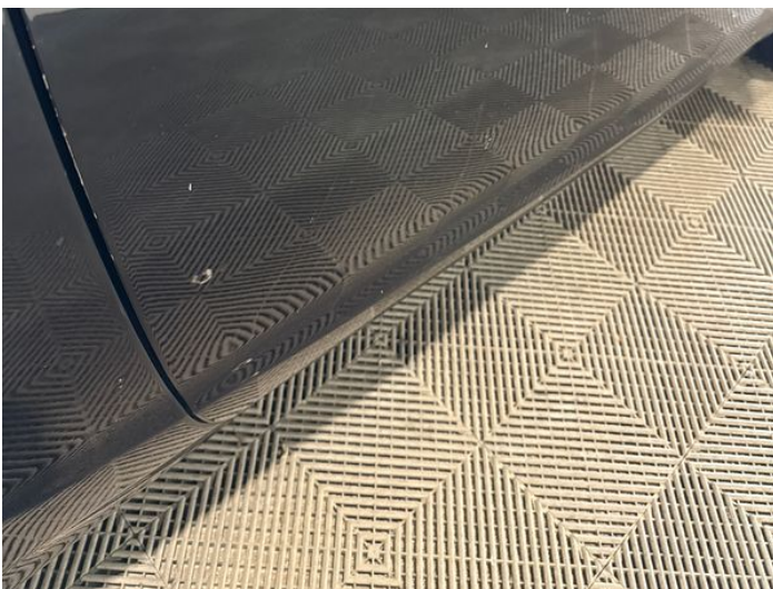
19: Door osf Scratched Over 25mm Thru Paint
