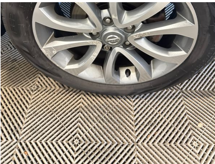
19: Wheel osf Scratched Over 50mm
