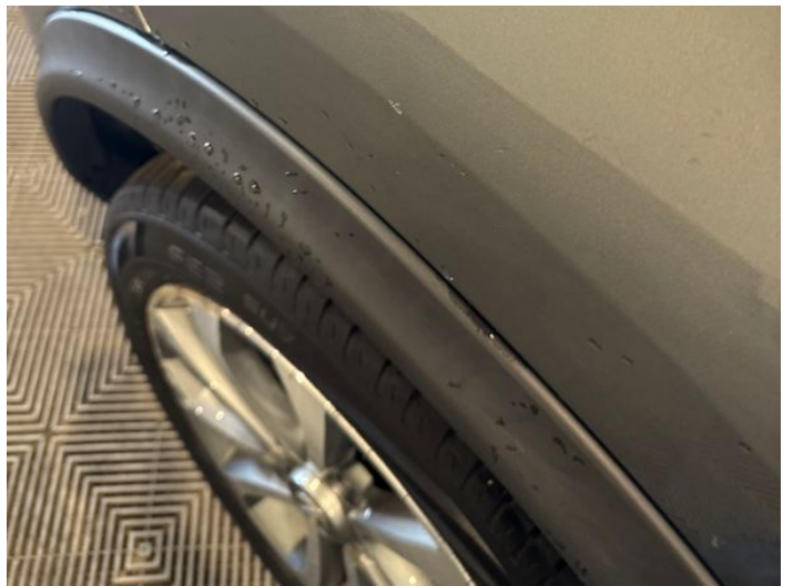
6: Wing nsf Scratched UpTo 25mm Thru Paint
