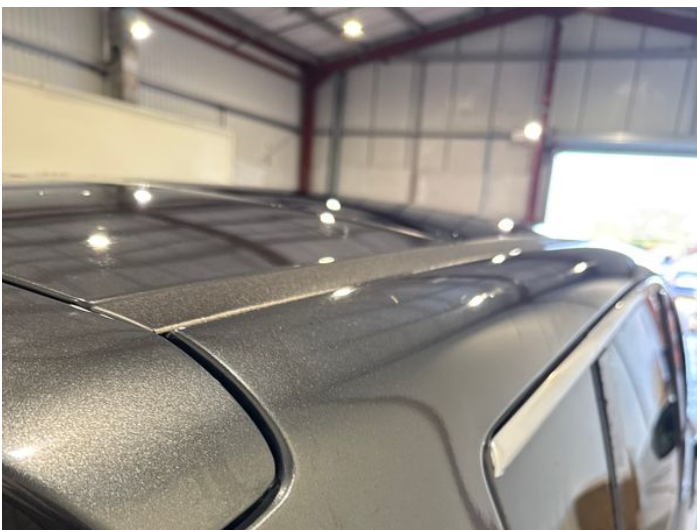
13: C Post os Dented Over 30mm
