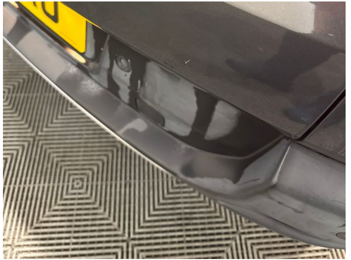
12: Tailgate Scratched UpTo 25mm Thru Paint
