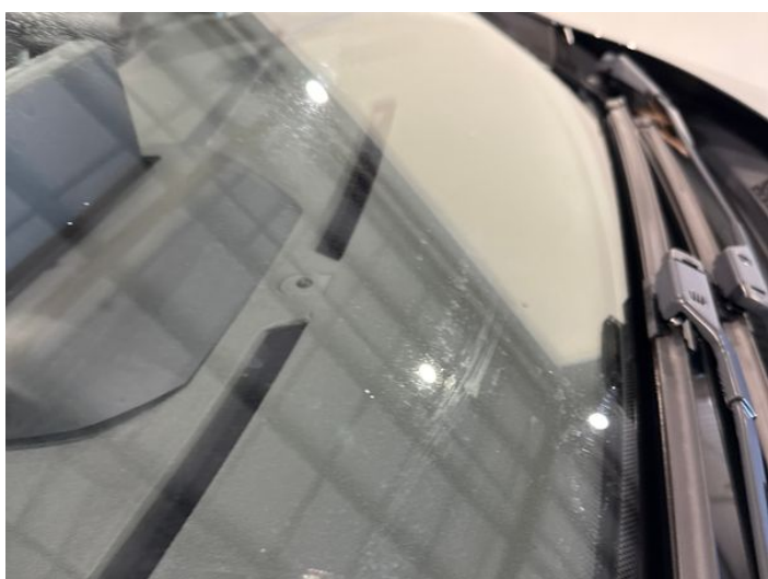
19: Screen Front Chipped UpTo 10mm
