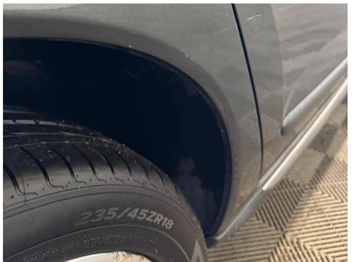
14: Qtr Panel osr Dented With Paint Damage
