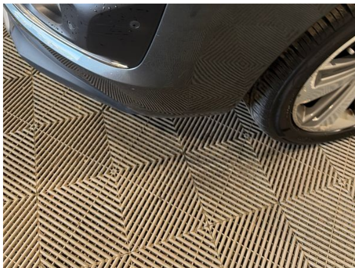
4: Bumper Front Scratched 25 to 100mm Thru Paint
