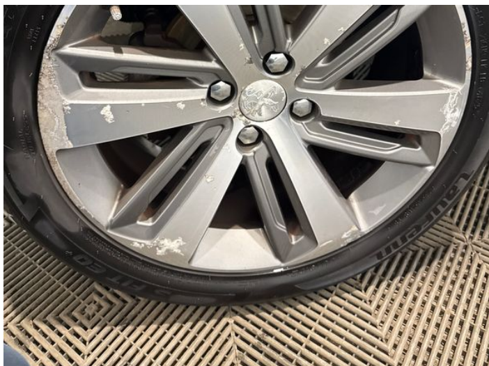
15: Wheel osr Scratched Over 50mm
