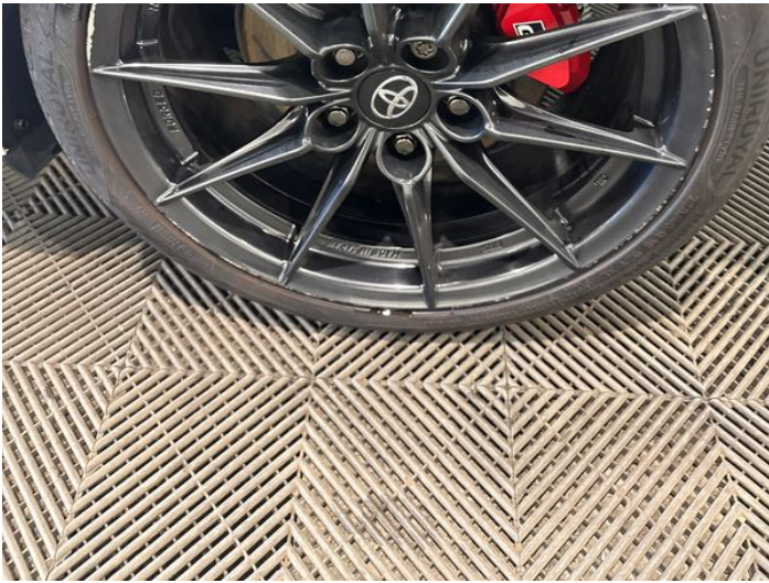
5: Wheel nsr Scratched Over 50mm
