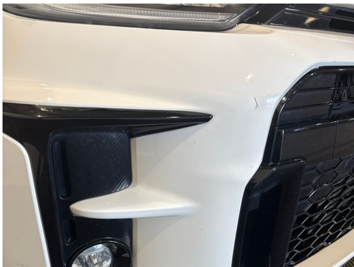
1: Bumper Front Dented With Paint Damage
