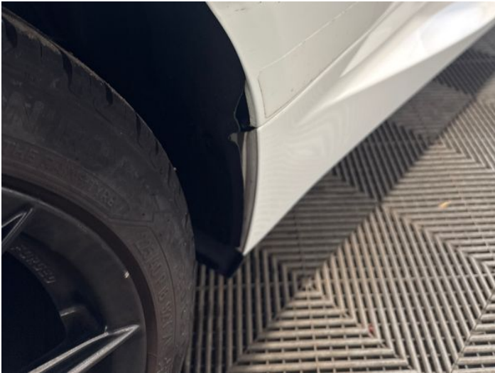
9: Qtr Panel osr Dented With Paint Damage
