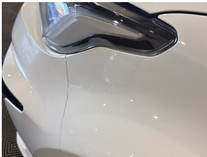
2: Wing nsf Chipped 1 To 5
