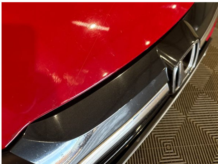
1: Bonnet Scratched Over 25mm Thru Paint
