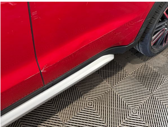
7: Door nsr Dented With Paint Damage
