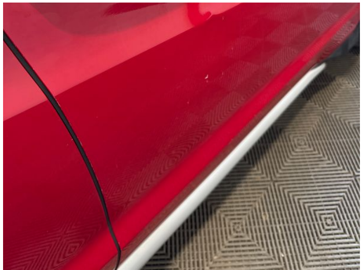
18: Door osf Dented With Paint Damage
