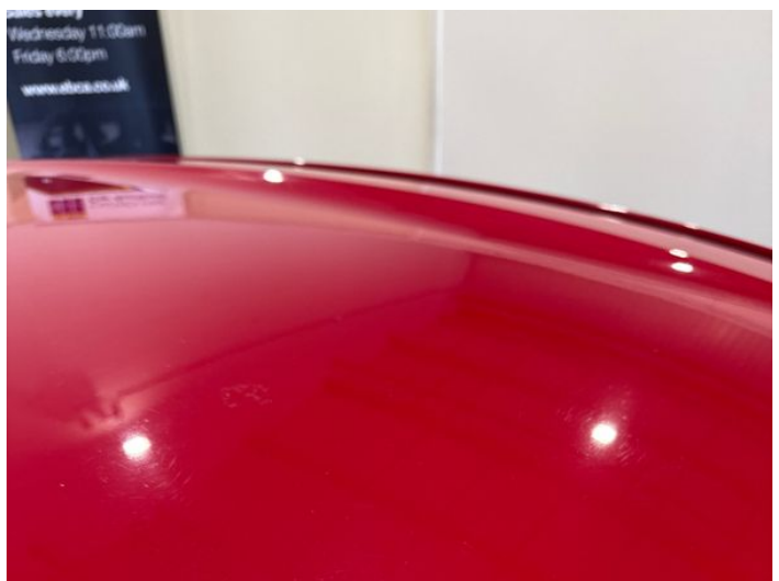
20: Roof Scratched Over 25mm Thru Paint
