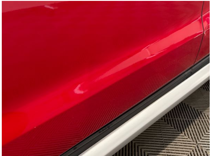
6: Door nsf Scratched Over 25mm Thru Paint
